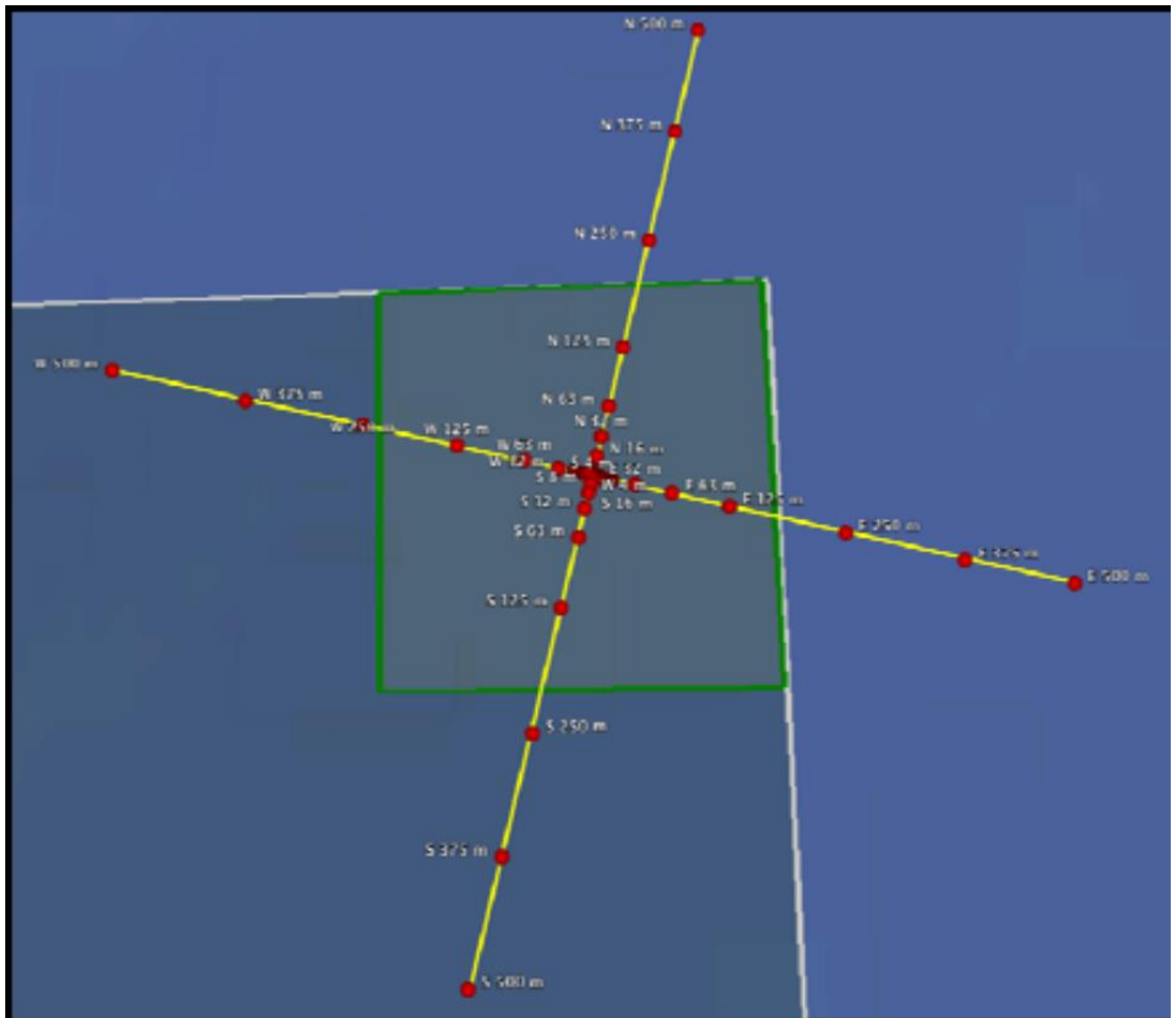
Figure 15: Prototypical EMF Survey Configuration
