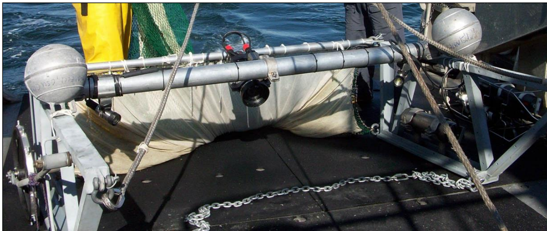
Figure 4: Beam trawl used for capturing juvenile groundfish and epibenthic invertebrates.
