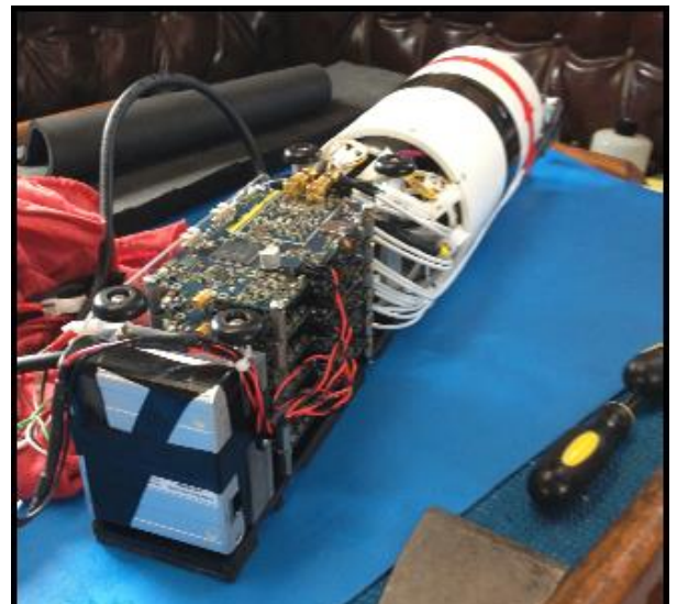
Figure 14: First Generation EMF measurement instrumentation.
