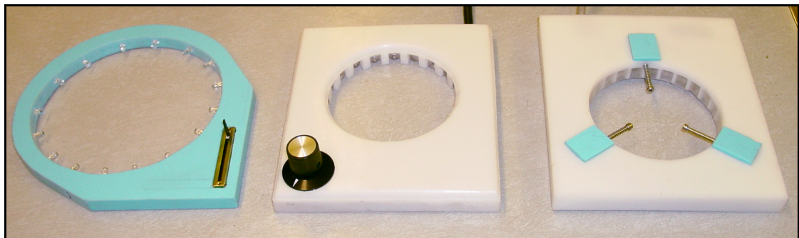
Figure 5 - Iterations of ring lighting shown chronologically from left to right
