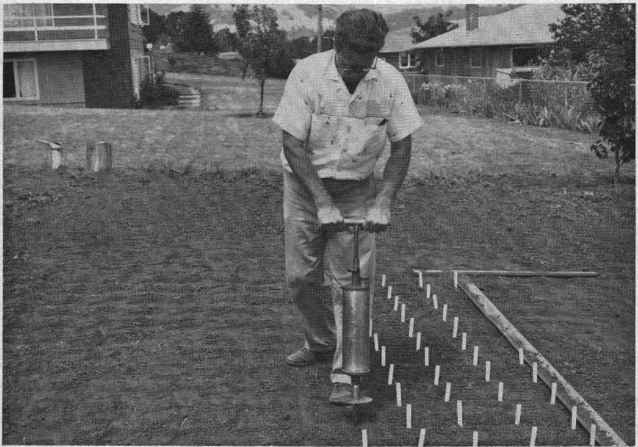
Figure 2. The area to be treated with a hand-operated injector is marked off in a regular grid pattern. Points where injections will be made are indicated by white markers.
