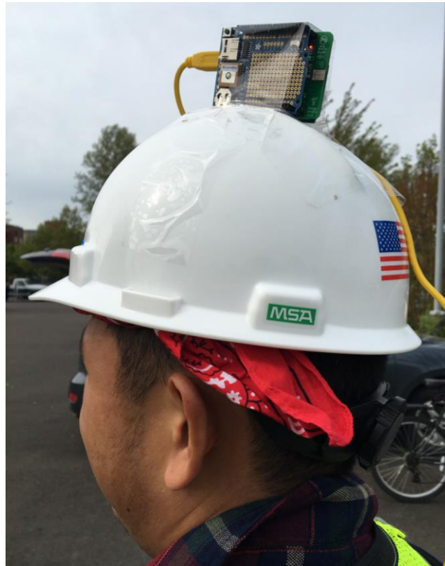
Figure 3.10: Hardware System Attached to Worker-on-Foot Hardhat
