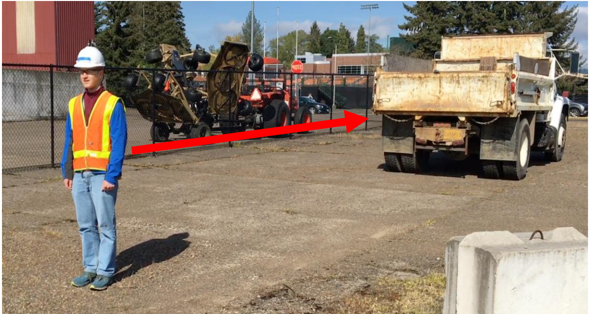
Figure 4.6: Enhanced Proximity Detection System Tested in Real-World Struck-By Equipment Case 1
