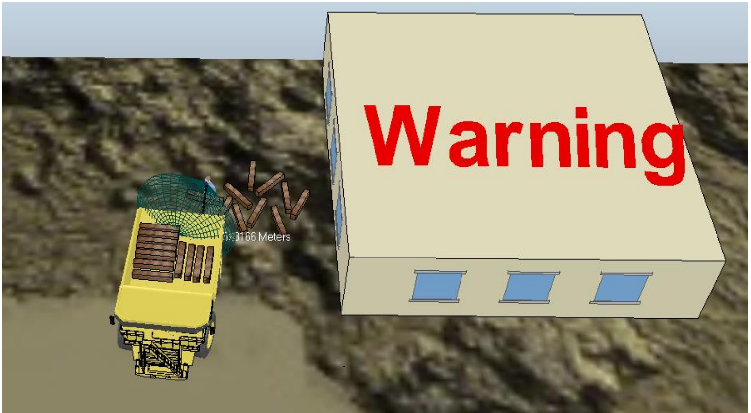
Figure 3.7: Warning Projected for Identified Hazardous On-Site Interaction
