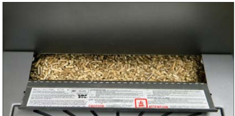
Figure 5.—Wood pellets in a pellet stove hopper.
