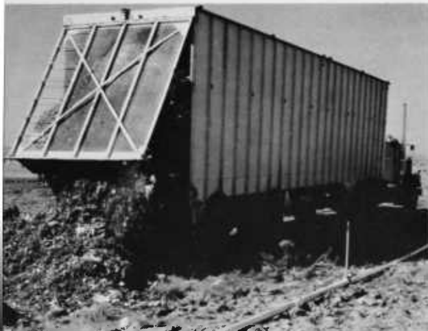
Shredded garbage goes into the soil at a rate of 400 tons per acre.
