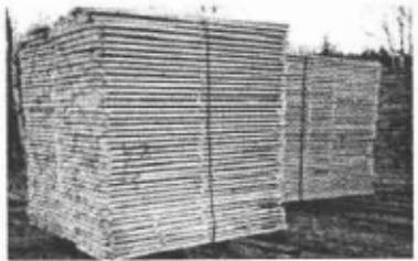
Lumber that we purchase already stickered will have different sticker and package sizes depending upon the producing mill. One of our suppliers uses a sticker size of 1" x 2" with a package size of 4' x 8'; one uses a sticker size of 5/8" x 4" with a package size of 5' x 7'; and one uses 3/4" x 2 1/2" strips with a package size of 5' x 5' and three lengths per package.
