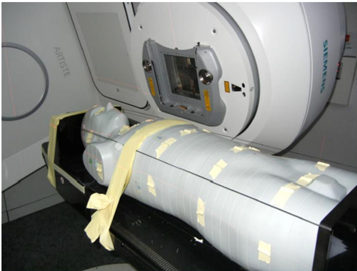
Figure 5. The anthropomorphic phantom in the treatment position for the measurement.
