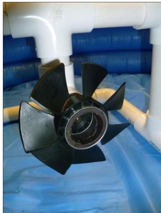
Figure 4-5: The tidal turbine demonstration setup in an inflatable wading pool. An electric sump pump is used to recirculate water, passing it over the turbine blades to simulate tidal flow. The generator is a small DC motor, and the power is calculated by measuring its output voltage and current using a handheld voltage meter.
