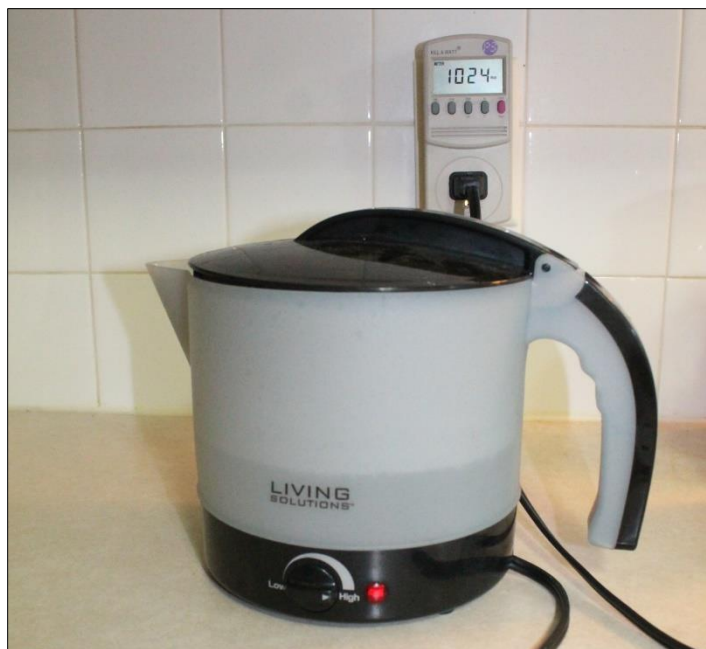
Figure 4-2: A Kill-A-Watt meter (background) being used to measure the power consumption of an electric hot pot (foreground). The hot pot plugs into the Kill-A-Watt, which displays power consumption in W.
