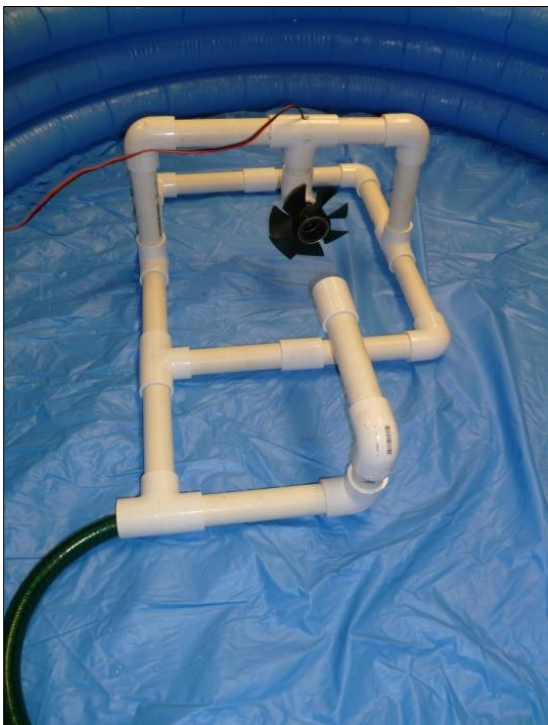
Figure 4-5: The tidal turbine demonstration setup in an inflatable wading pool. An electric sump pump is used to recirculate water, passing it over the turbine blades to simulate tidal flow. The generator is a small DC motor, and the power is calculated by measuring its output voltage and current using a handheld voltage meter.
