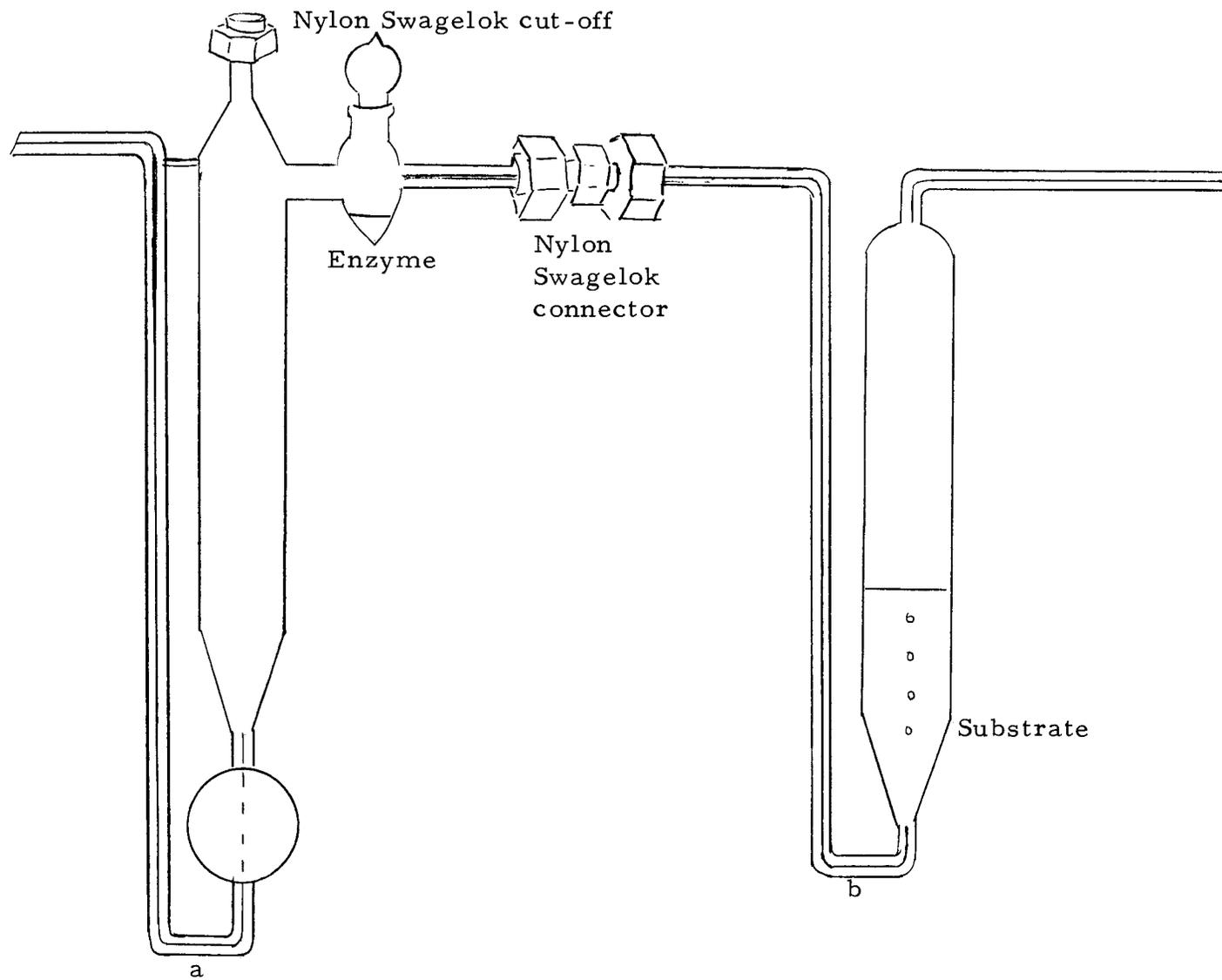
Figure 3. Diagrams of a-enzyme-reaction vessel and b-substrate vessel.
