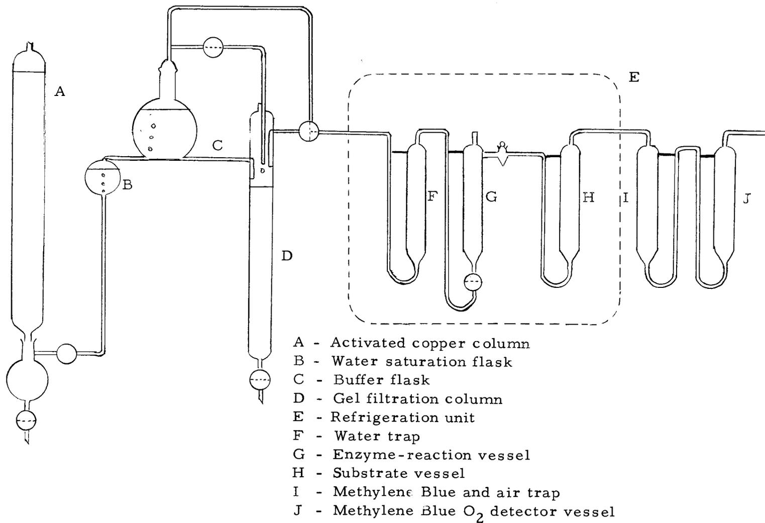
Figure 2. Diagram of system for running enzyme reactions in an O<sub>2</sub>-free N<sub>2</sub> atmosphere.
