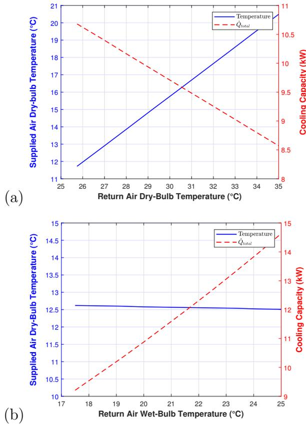
Figure 3: Membrane system supplied air-dry bulb temperature and total cooling capacity versus (a) indoor return air dry-bulb and (b) indoor return air wet-bulb
