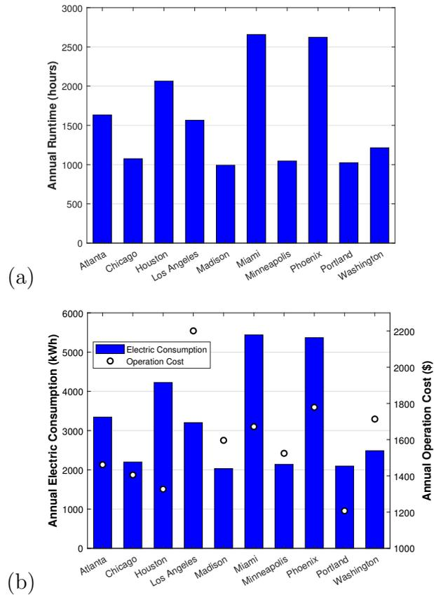
Figure 4: (a) Membrane system annual run time, (b) Membrane system annual electric consumption and costs
