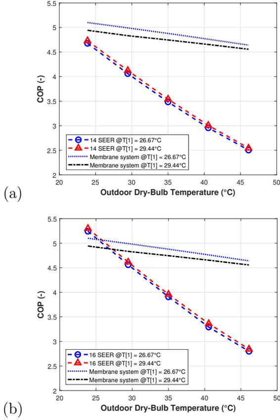
Figure 5: Membrane and vapor compression system COP versus outdoor dry-bulb temperature at outdoor wet-bulb of 23.69°C and indoor wet-bulb of 21.67°C for (a) 14 SEER vapor compression system and (b) 16 SEER vapor compression system
