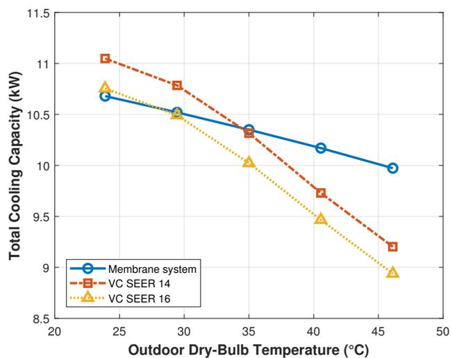
Figure 6: Membrane and vapor compression system total cooling capacity versus outdoor dry-bulb temperature at outdoor wet-bulb of 23.69°C and fixed indoor return air conditions of 26.67°C dry-bulb and 19.4°C wet-bulb
