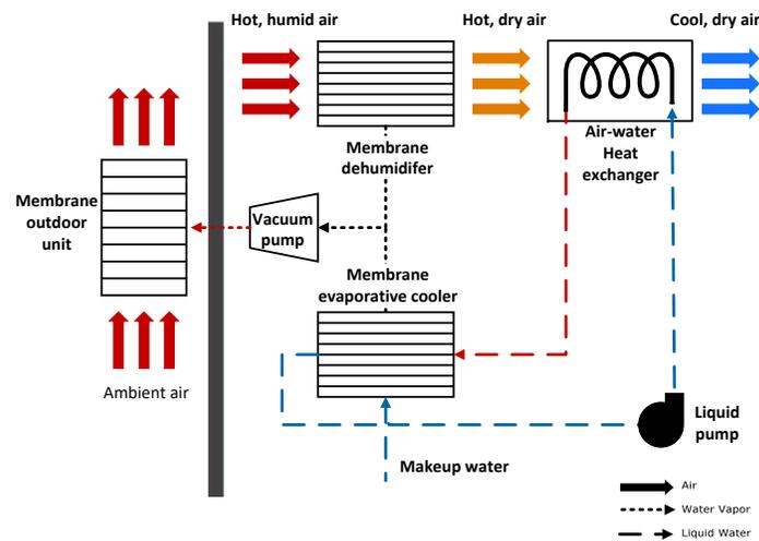
Figure 1: Schematic of membrane heat pump system with labeled state points
