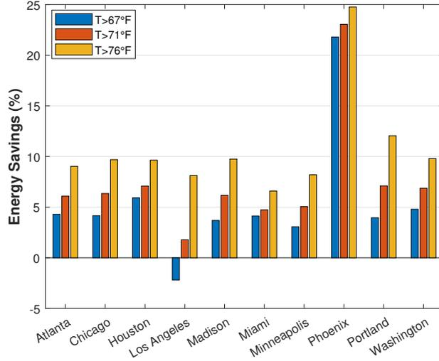
Figure 9: Annual energy savings of membrane system versus 16 SEER vapor compression system
