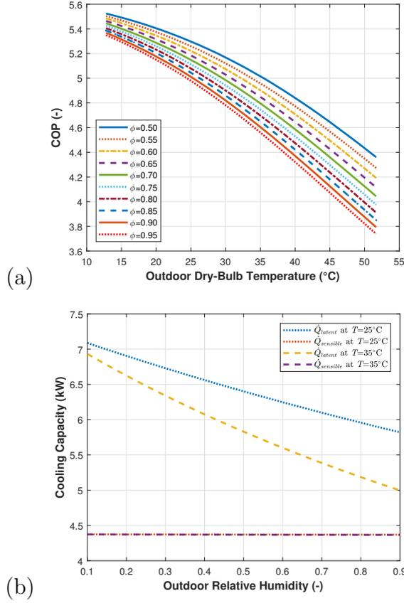
Figure 2: (a) Membrane heat pump system COP at different ambient conditions and (b) Membrane system total, latent and sensible cooling capacity at different ambient conditions
