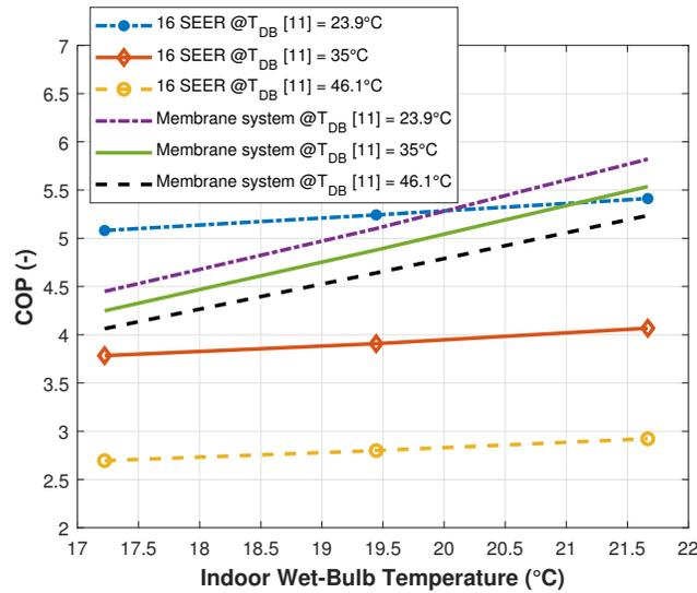
Figure 7: Membrane and vapor compression system COP versus indoor return air wet-bulb temperature at fixed outdoor conditions of 26.67°C dry-bulb and 23.69°C wet-bulb
