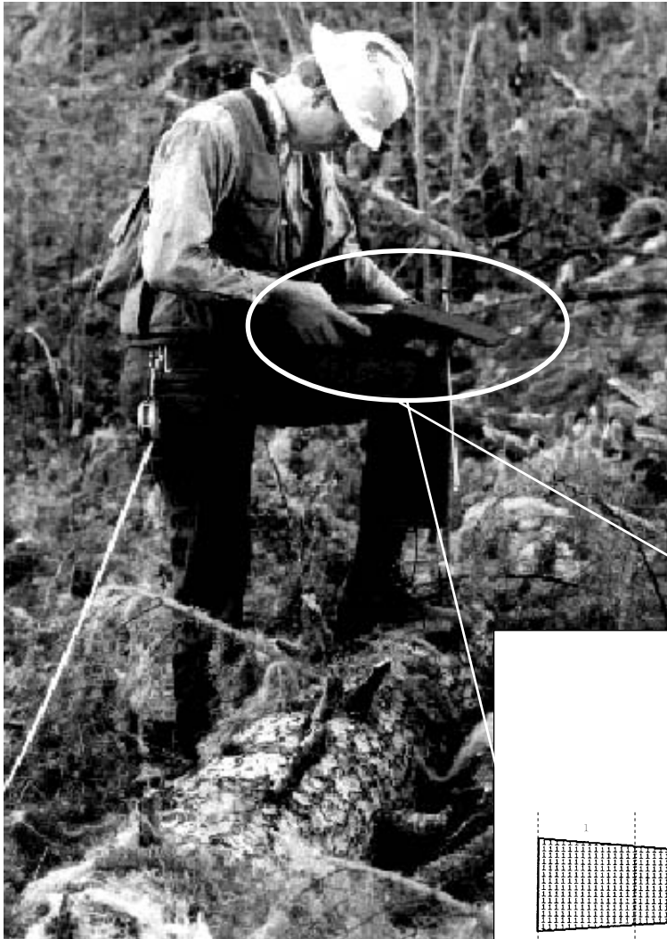
Figure 2. Field data being entered into a handheld computer by a Log Quality Technician. Inset: a typical display sequence.
