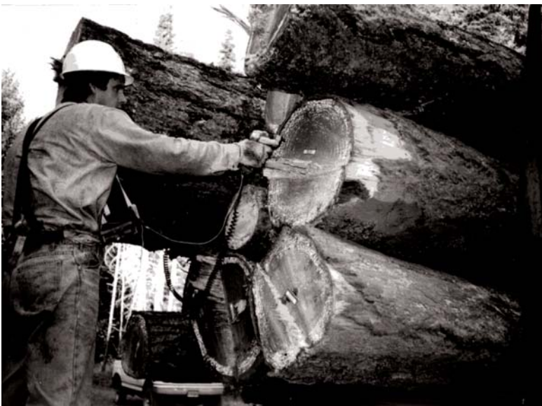
Figure 5. A bar-code scanner being used on a truckload of logs.
