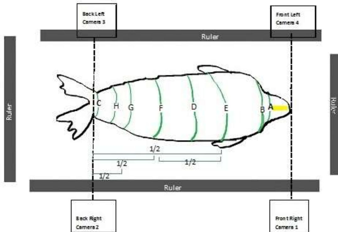
**Figure 1.** Photogrammetry set up
