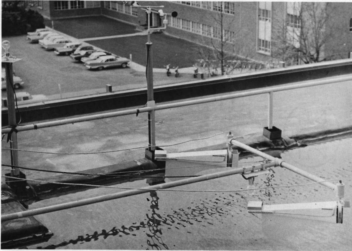
Figure 9. The new total hemispherical radiometers mounted for rooftop tests. On the boom is also mounted an inverted Eppley pyranometer. In the background are the upright Eppley pyranometer (left) and the wind measuring equipment (center).
