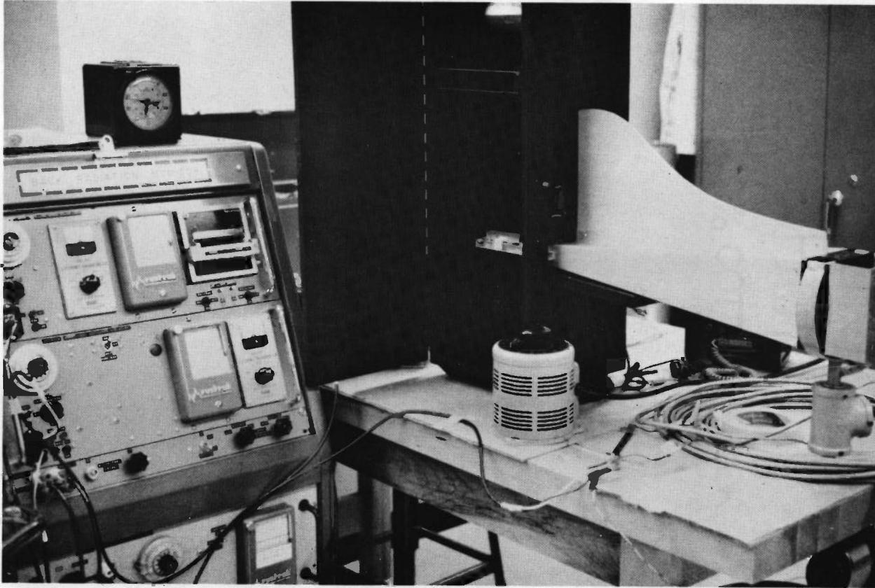
Figure 8. Test box with total hemispherical radiometer in position to determine its time constant.
