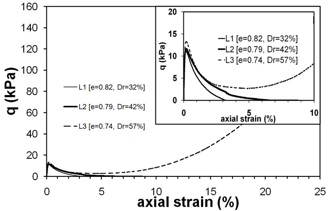
Fig. 2.5. Evolution of  $q_{\text{peak}}$  and the instability line for a loose silty sand due to densification.
