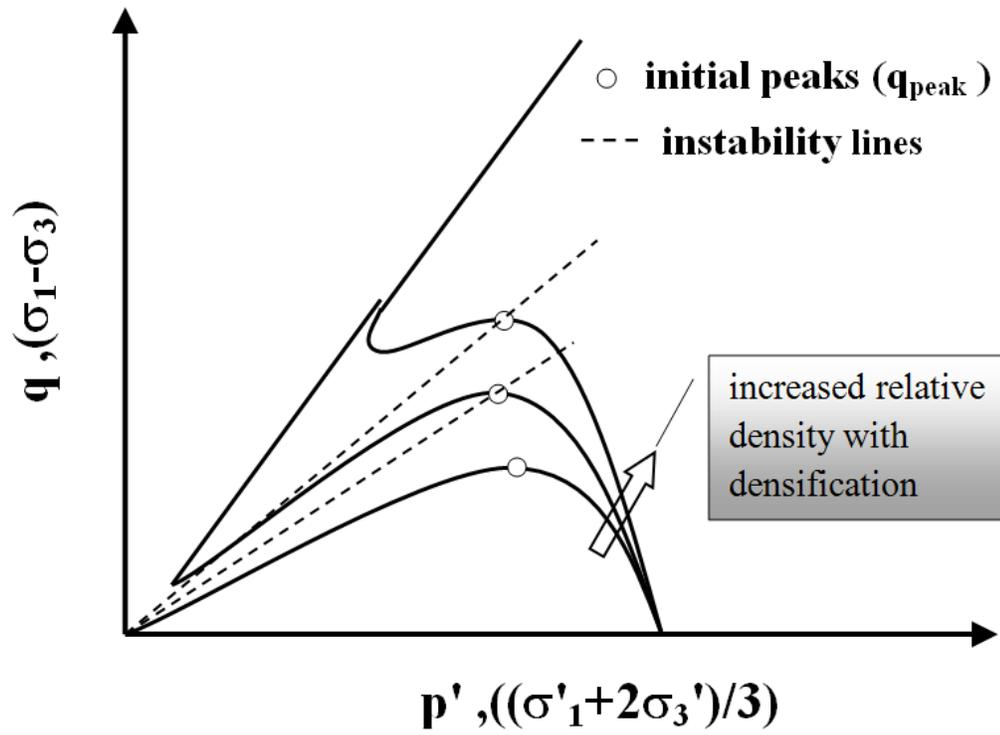
Fig. 2.6. Normalized initial peak principal stress difference versus relative density for different silty sands prepared with moist tamping.
