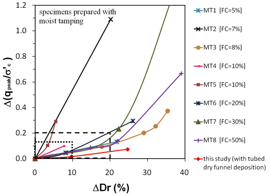
Fig. 2.8. Change in normalized initial peak principal stress difference versus change in relative density for dry funnel specimens.
