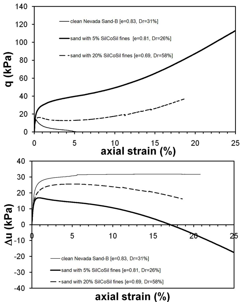
Fig. 4.6 a) Principal stress difference versus axial strain response; b) change of excess pore pressure with axial strain for Nevada Sand-B with different percentages of Potsdam fines at 30 kPa confining stress.
