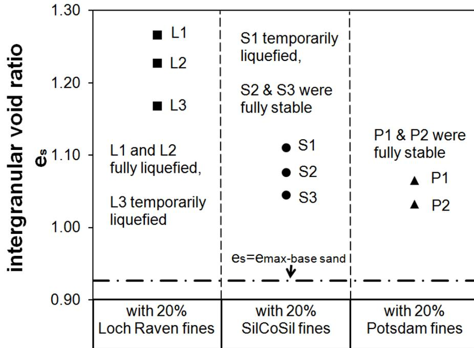
Fig. 3.9. Change of void ratio and liquefaction potential for tested specimens.
