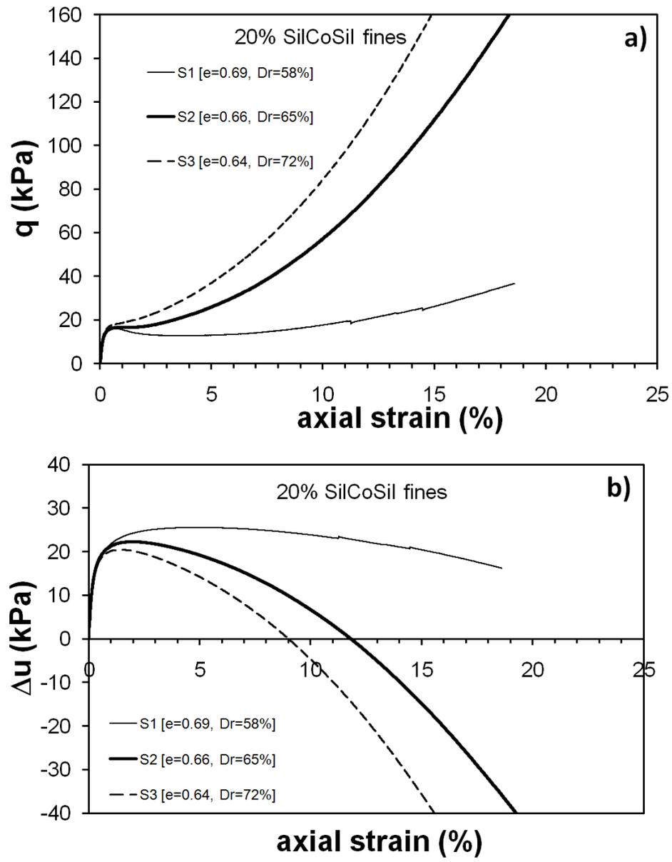
Fig. 3.6. a) Principal stress difference versus axial strain response; b) change of excess pore pressure with axial strain for Nevada Sand-B with 20% Potsdam fines at 30 kPa confining stress.
