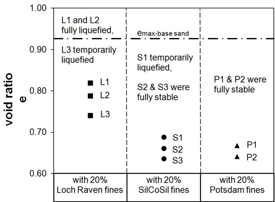
Fig. 3.10. Change of relative density and liquefaction potential for tested specimens.
