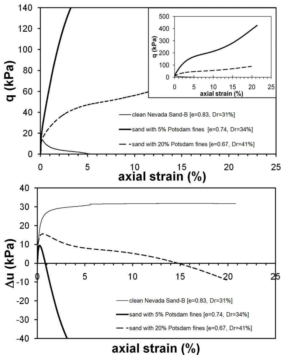
Fig. 4.7. Change of void ratio and liquefaction potential with different fines contents and silts for tested specimens.
