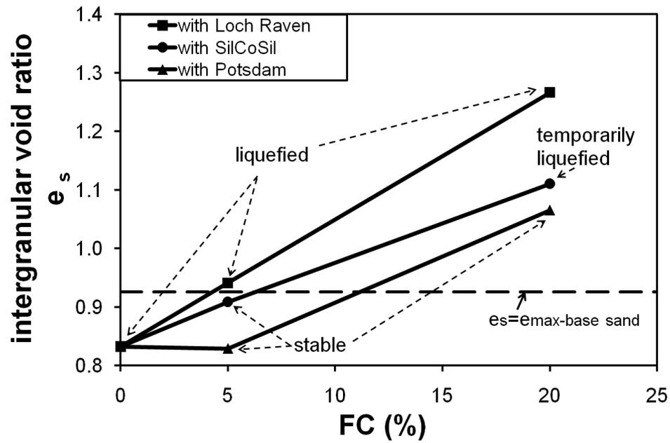
Fig. 4.9. Change of relative density and liquefaction potential with different fines contents and silts for tested specimens.
