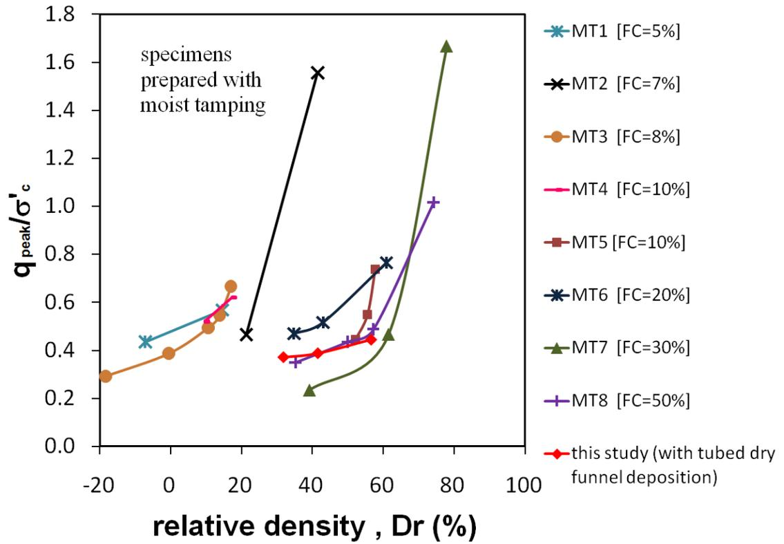
Fig. 2.7. Change in normalized initial peak principal stress difference versus change in relative density for moist tamped specimens.
