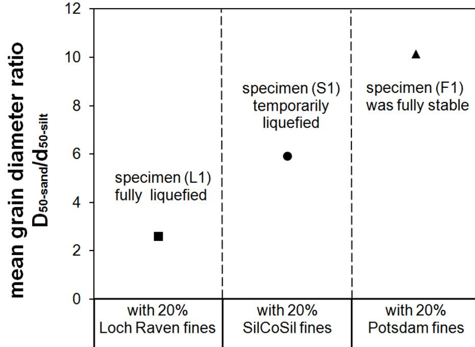
Fig. 3.8. Change of intergranular void ratio and liquefaction potential for tested specimens.
