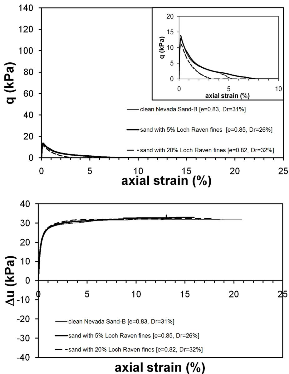
Fig. 4.5 a) Principal stress difference versus axial strain response; b) change of excess pore pressure with axial strain for Nevada Sand-B with different percentages of SilCoSil fines at 30 kPa confining stress.
