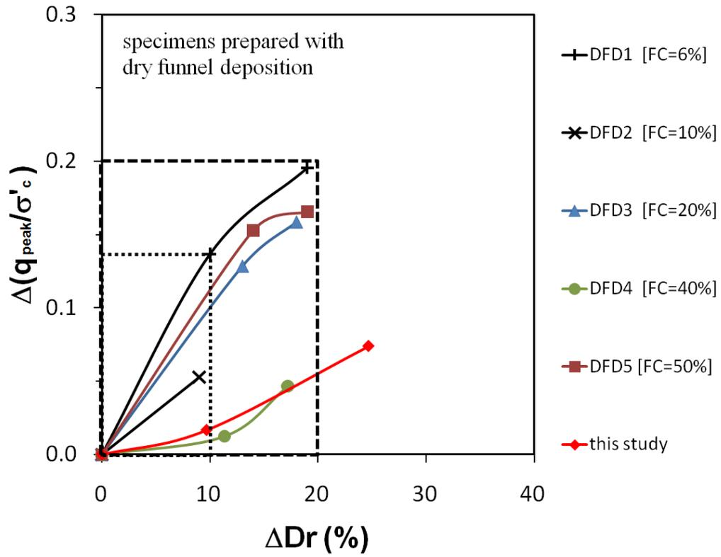
Fig. 2.9. Change in normalized initial peak principal stress difference versus change in relative density for slurry deposited specimens.
