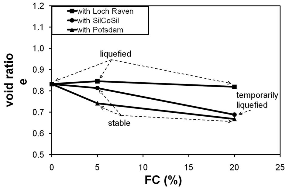
Fig. 4.8. Change of intergranular void ratio and liquefaction potential with different fines contents and silts for tested specimens.
