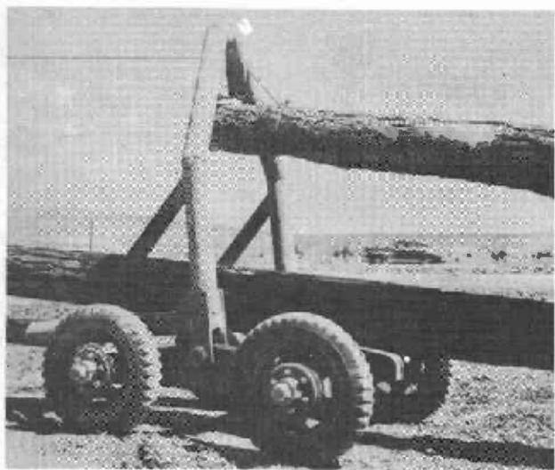
Figure 2.--Loading log over rear bunk.
