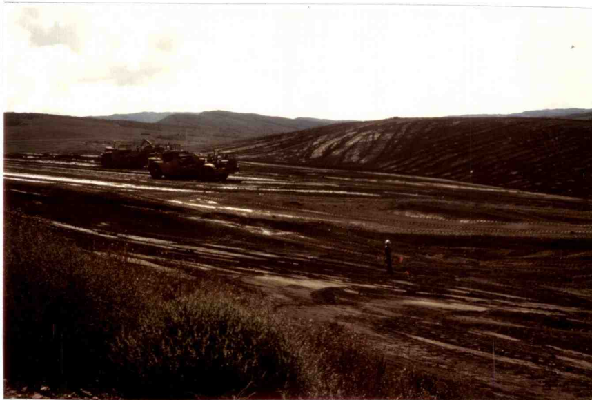
Figure 6. Paddlewheel scrapers removing topsoil at Energy 3 Mine. Source: Photo by author.
