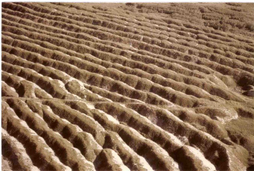
Figure 3. Upgraded spoils at the Edna Mine stockpiled between 1947 and 1962. Notice the road across the spoil piles which are approximately twelve meters (40 feet) high. Source: Photo by author.
