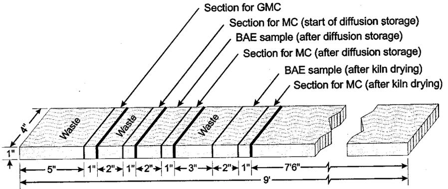
**FIGURE 2.** Sampling diagram for each board.
