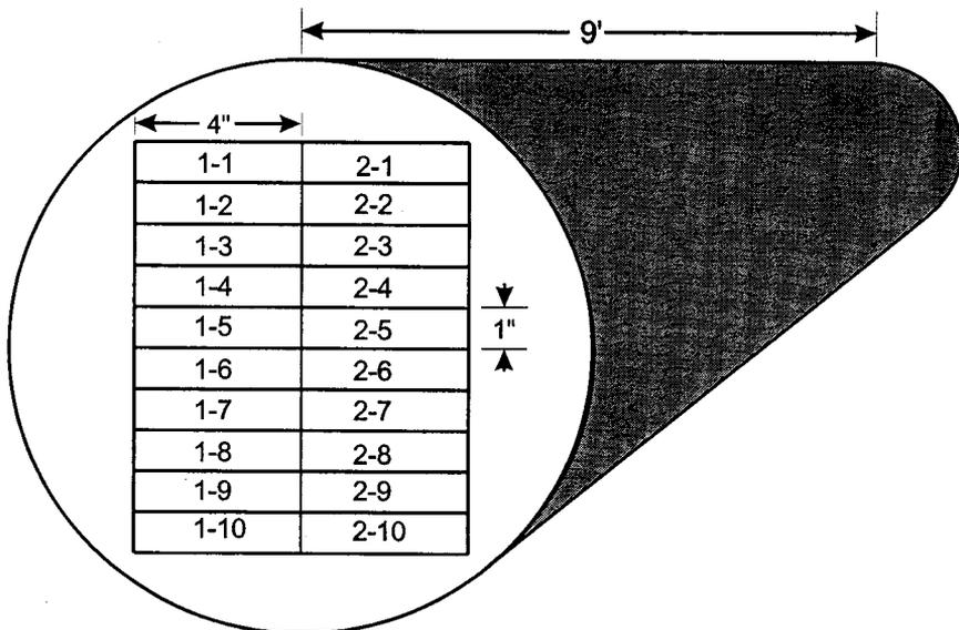
**FIGURE 1.** Locations of 10 sample boards per cant and two cants per log.
