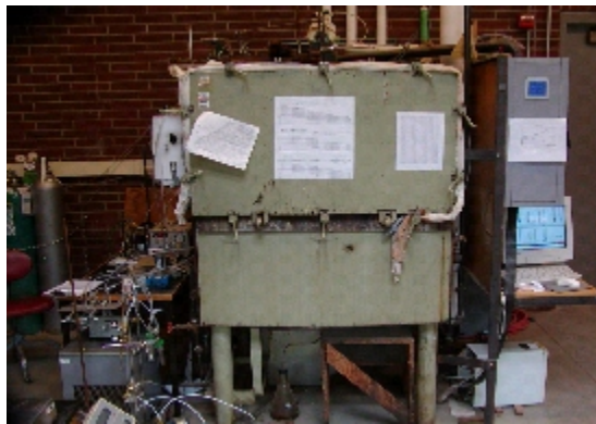
FIGURE 1. Schematic of kiln and sampling system.
