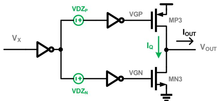
Figure 2.9: Schematic of a ringamp
