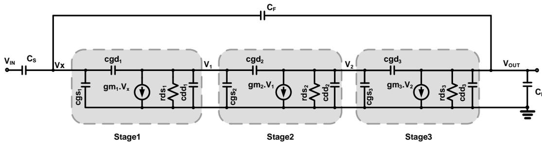
Figure 2.18: RC model for initial large-signal step response. (a) Positive output step
