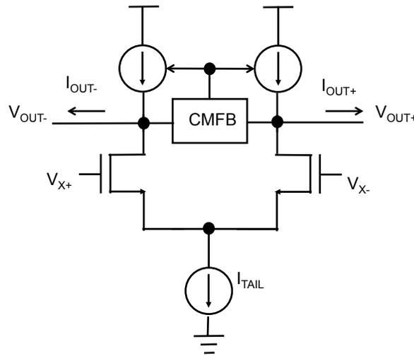
Figure 2.3: Schematic of a single-stage OTA
