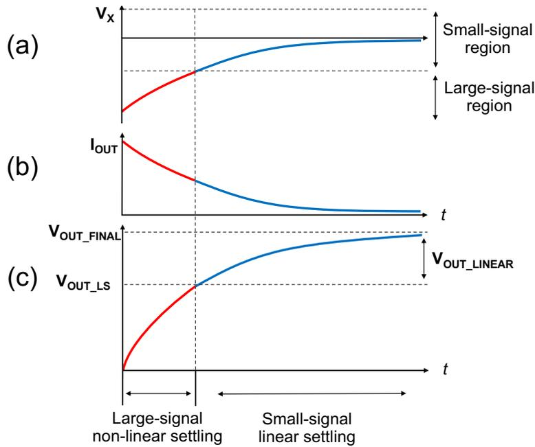
Figure 2.8: IBA transient response (a) Differential virtual ground node voltage (b) Differential output current (c) Differential Output Voltage
