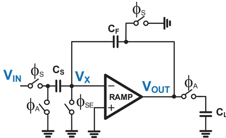
Figure 3.4: Switched capacitor amplifier setup
