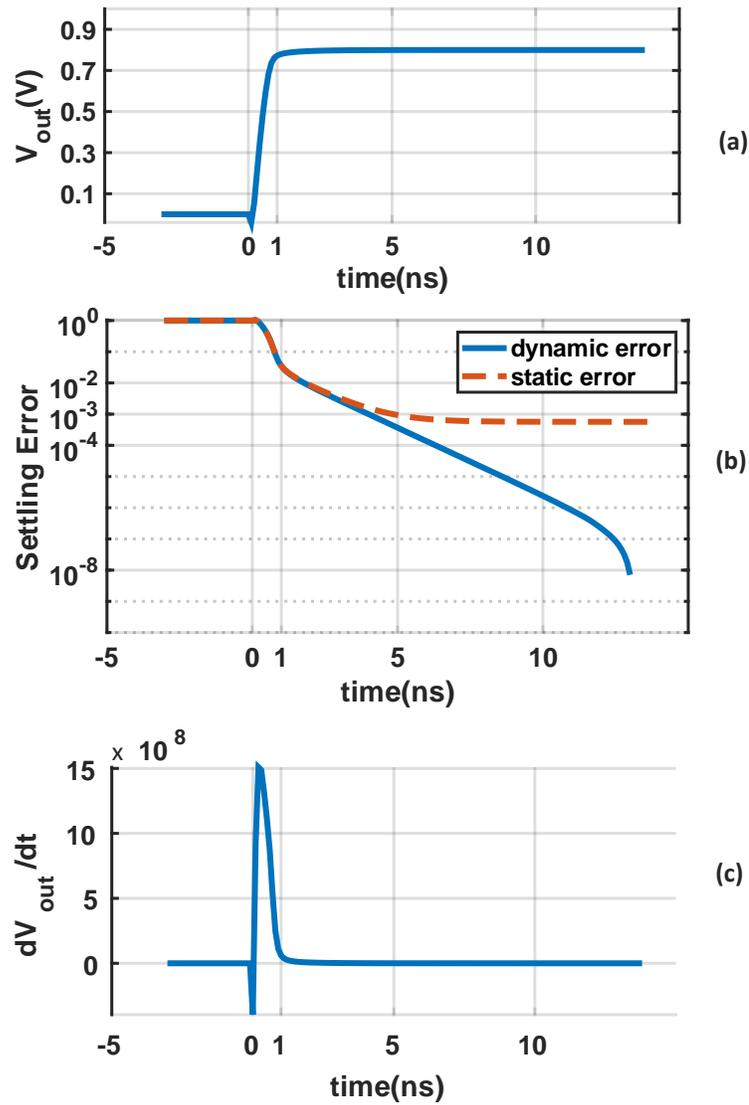
Figure 2.22: Settling response of the ring-amplifier. (a) Differential output voltage step of 800mV (b) Dynamic and static errors illustrating the fast large-signal slope and slow small-signal slope sections (c) Derivative of output voltage representing the exponential decay of current through the load capacitor
