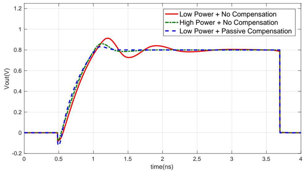
Figure 4.5: Transient response with and without passive compensation for large signal ringing
