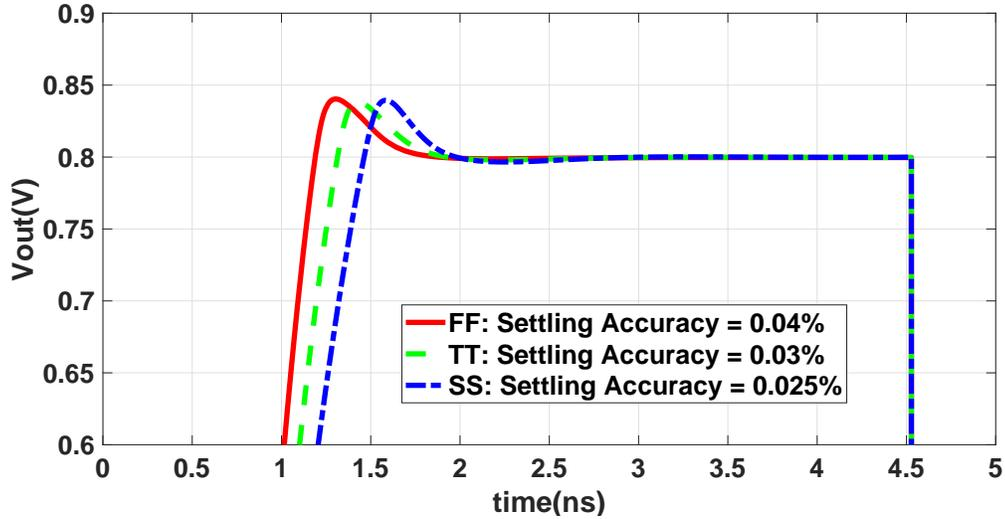
Figure 3.7: Transient response with the deadzone regulation circuit
