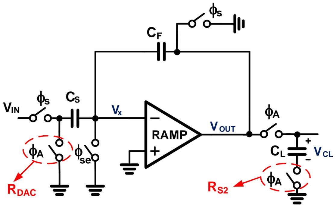
Figure 4.1: Passive compensation of ring amplifier using switches in the feedback network
