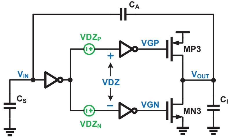
Figure 3.1: Traditional ringamp in a switched capacitor negative feedback
