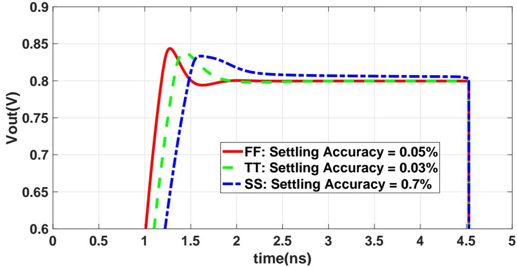
Figure 3.5: Transient response with fixed deadzone bias
