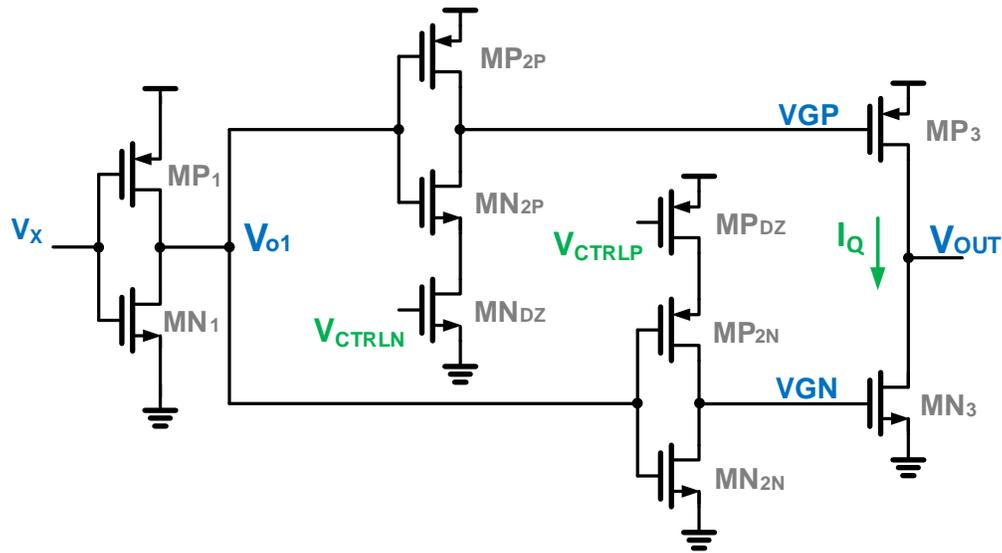
Figure 3.3: Ringamp using current starved inverters for deadzone biasing.
