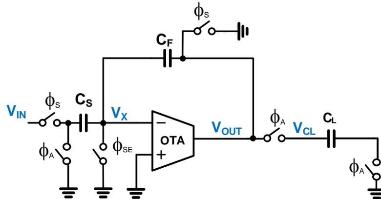
Figure 2.1: Switched capacitor amplifier setup
