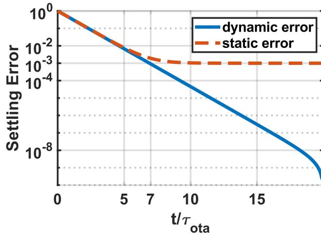
Figure 2.17: Dynamic settling error and overall settling error in log scale
