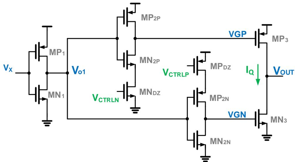
Figure 2.21: Current-starved-inverter based ring-amplifier used for design example. (Single-ended schematic shown for simplicity. First-stage biased with tail current sources for differential implementation)
