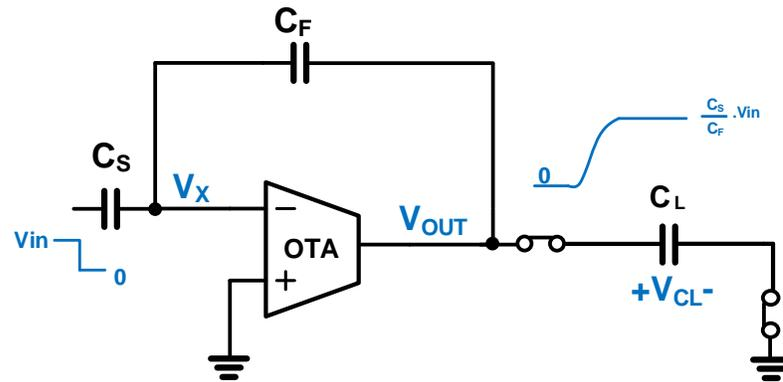
Figure 2.2: Charge transfer as step response
