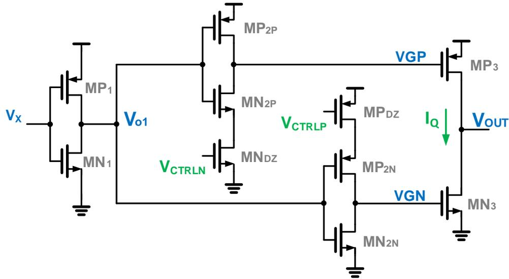
Figure 4.2: Ring amplifier using current-starved inverters. (Single-ended schematic shown for simplicity. First-stage biased with tail current sources for differential implementation)
