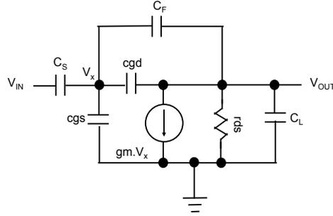
Figure 2.14: Small-signal model of an OTA during the charge transfer phase of a SC amplifier
