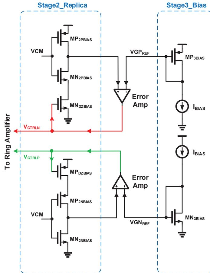
Figure 3.6: Deadzone regulation circuit for current starved inverter based ring amplifier
