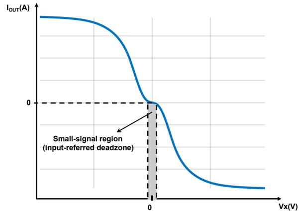
Figure 2.10: I-V characteristics of a ringamp
