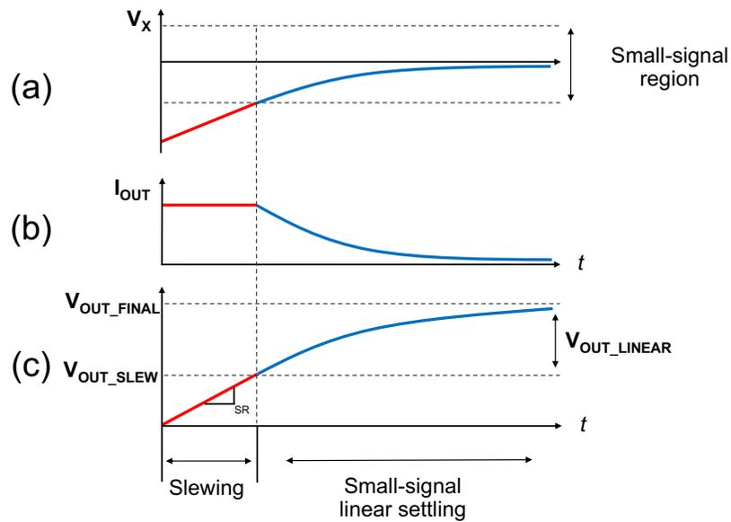
Figure 2.5: OTA transient response (a) Virtual ground node  $V_x$  (b) Differential output current  $I_{Out}$  (c) Differential output voltage
