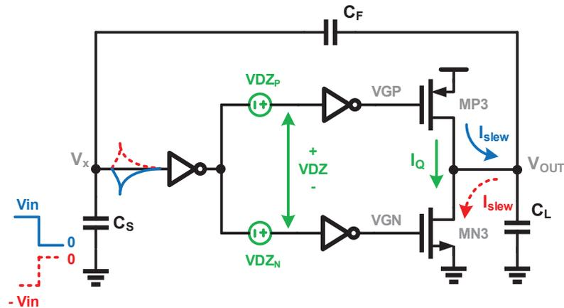
Figure 1.1: Ringamp: Basic structure and operation
