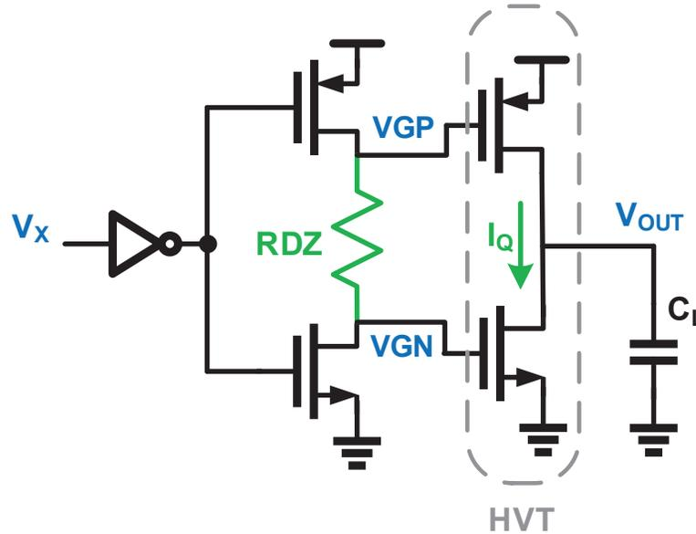
Figure 3.2: Ringamp using a resistor for deadzone biasing
