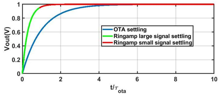
Figure 2.20: Settling response for a ringamp compared to single-stage OTA (y-axis normalized to final value)
