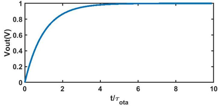
Figure 2.16: Settling response for a single-stage OTA (y-axis normalized to final value)
