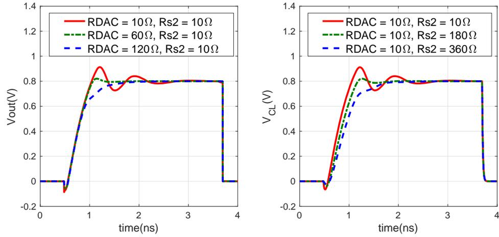
Figure 4.4: Transient response with large signal ringing. (a) Effect of  $R_{DAC}$  on the output voltage,  $V_{out}$ . (b) Effect of  $R_{S2}$  on the voltage across the load capacitor,  $V_{CL}$
