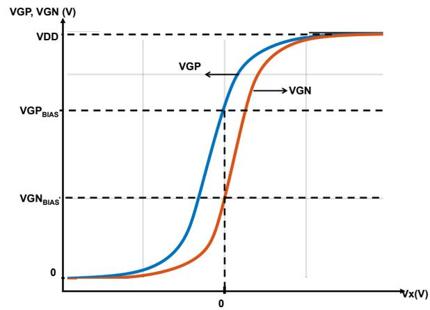
Figure 2.11: V-V transfer characteristics of the first two stages of a ringamp
