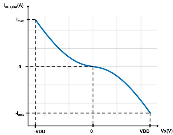
Figure 2.7: I-V characteristics of a single-stage IBA
