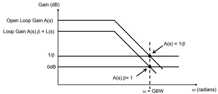
Figure 2.15: Bode plot showing loop-gain and GBW
