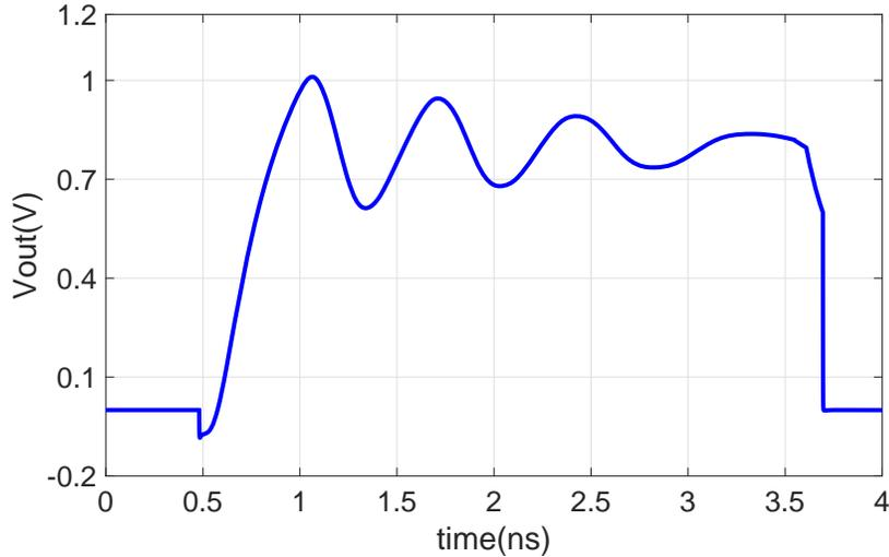
Figure 4.3: Large signal ringing even with a phase margin of 70 degrees from ac response
