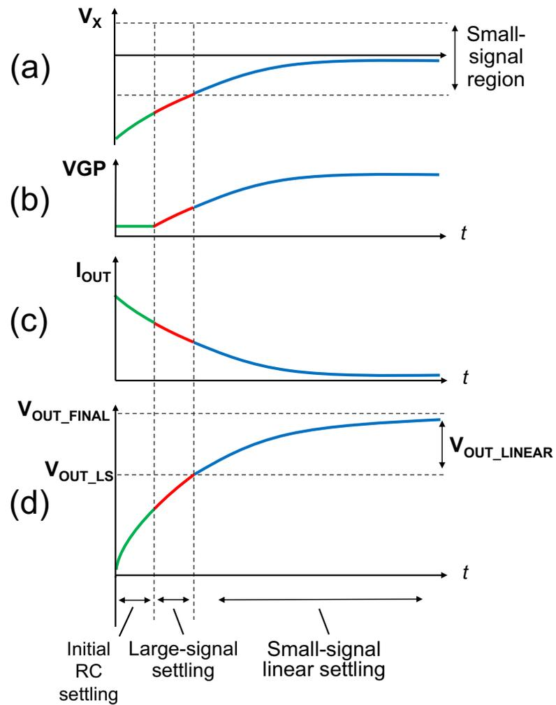
Figure 2.12: Ringamp transient response (a) Differential virtual ground node (b) Single-ended output voltage of the second-stage (c) Differential output current (d) Differential Output Voltage
