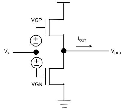
Figure 2.6: Schematic of a single-stage class-AB inverter-based amplifier (IBA)
