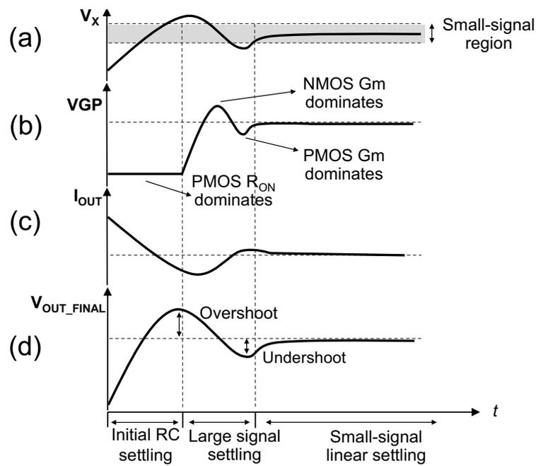
Figure 2.13: Ringamp transient response with overshoot (a) Differential virtual ground node (b) Single-ended output voltage of the second-stage (b) Differential output current (c) Differential Output Voltage
