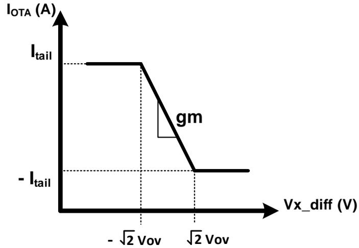
Figure 2.4: I-V characteristics of a single-stage OTA
