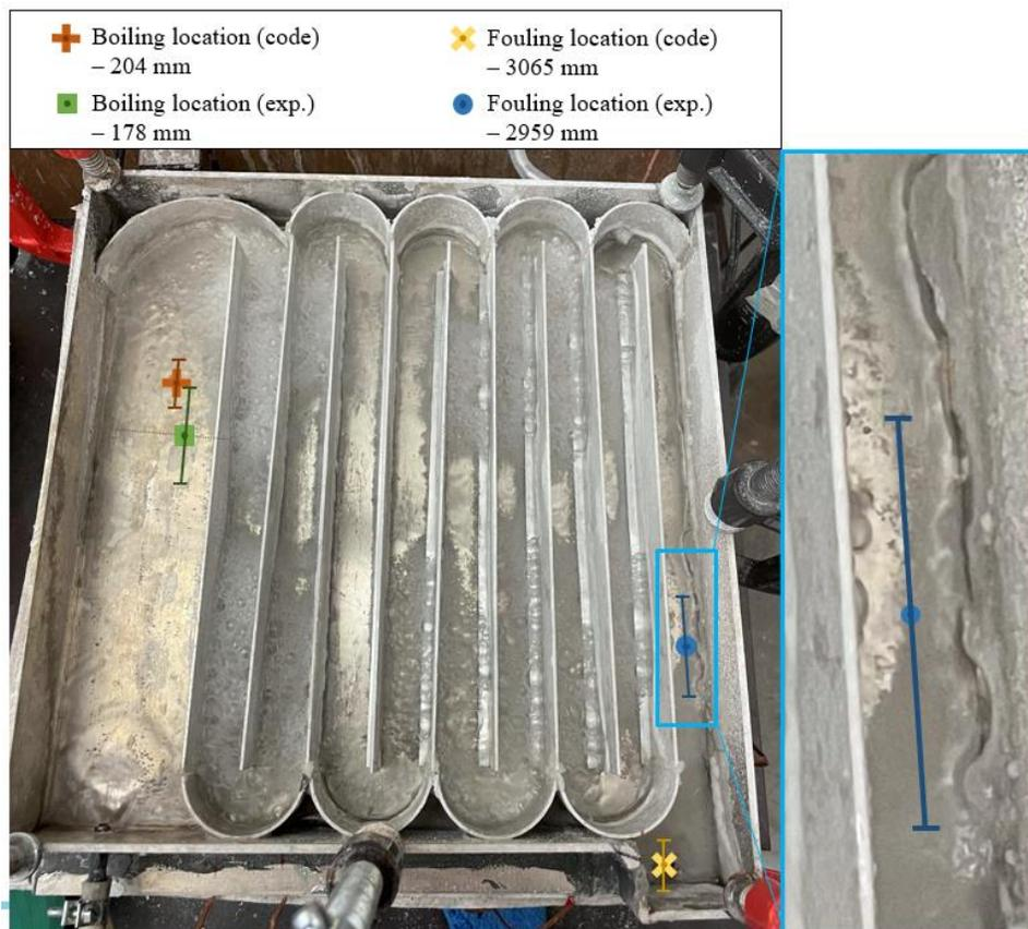
**Figure 4.2** Boiling and fouling locations of experiment and code estimates for 2.8 g/s 10% NaCl and 10% KCl saline
