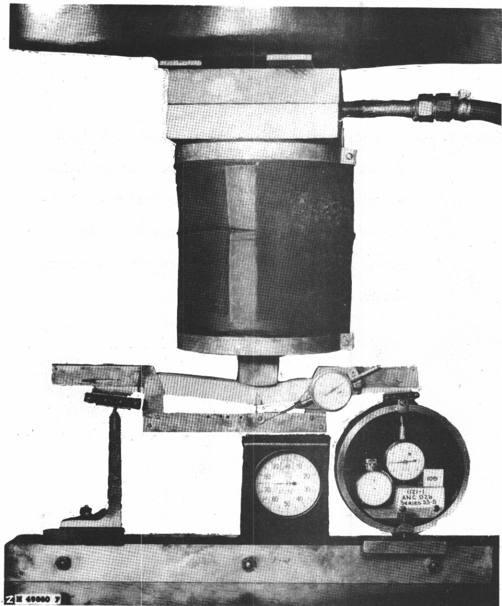
Figure 8.--The effect of rate of load application on the ultimate compressive strength of small clear Sitka spruce compression-parallel-to-grain specimens.
