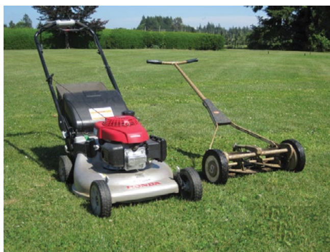
Figure 8: Rotary mowers (above left), while durable, typically cannot be set to a height below 1 inch. Push reel mowers (above right) typically cannot be set higher than 2 inches.
