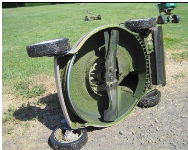
Figure 9. The double blade pattern of a mulching mower is designed to thoroughly mulch grass clippings.
