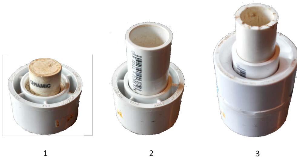
*Figure 2: 1 shows the ceramic rod sitting in the end cap within the first bushing. 2 Shows the addition of the coupler onto the ceramic rod. 3 Shows the addition of the second bushing as well as the soil holder/sampler inserted into the bushing. The entire assembly is then loaded into a 500 ml centrifuge vial holder.*
