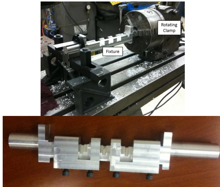
Figure 25: Tube machining fixture; setup on a vertical milling machine (top), fixture and clamps (bottom)
