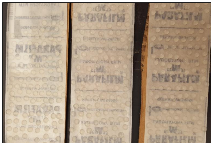
Figure 8. Agarose beads cooling after dropping onto the wax paper using the syringe pump.
