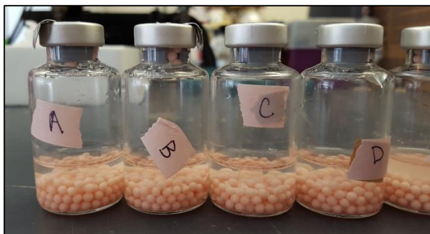
Figure 9. OB3b immobilized in alginate beads in batch reactor vials. All vials contain hydrogel beads, media, and a headspace of air with methane additions.
