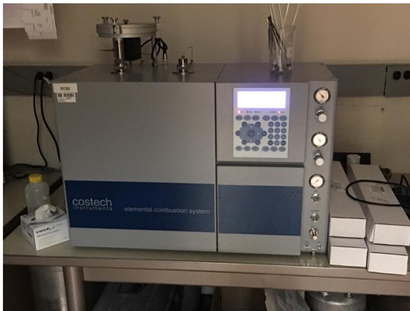
Figure 3-4: Costech ECS 4010 CHNS-O Elemental Analyzer
