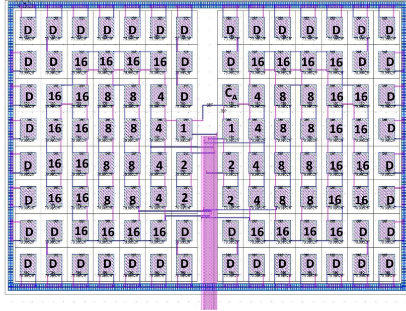
Fig. 3.8 Capacitive DAC array floorplan and layout.
