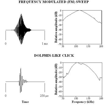
FIG. 2. Waveforms and spectrograms of the incident sonar signals.
