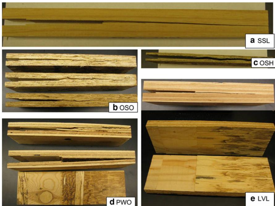
**Fig. 4** Crack propagation failure modes for various materials. **a** Solid sawn lumber (SSL); **b** One-inch OSB (OSO); **c** Half-inch OSB (OSH); **d** One-inch plywood (PWO); **e** LVL
