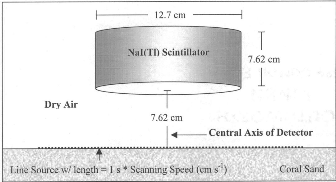
**Figure 2.** Model geometry for MCNP4b investigation of scanning detection efficiency of a 12.7 cm x 7.62 cm NaI(Tl) scintillator.
