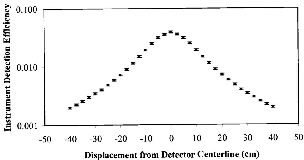
**Figure 6.** Experimentally determined 12.5 cm x 7.62 cm NaI(Tl) scintillator static detection efficiency of 661.67 keV photons as a function of position from the central axis of the detector. Error bars represent the 95% confidence interval, based on propagating the errors in counting statistics and in the measured source emission rate.
