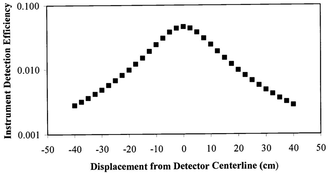
**Figure 4.** MCNP4b simulated 12.5 cm x 7.62 cm NaI(Tl) scintillator theoretical static detection efficiency for 661.67 keV photons as a function of position from the central axis of the detector.
