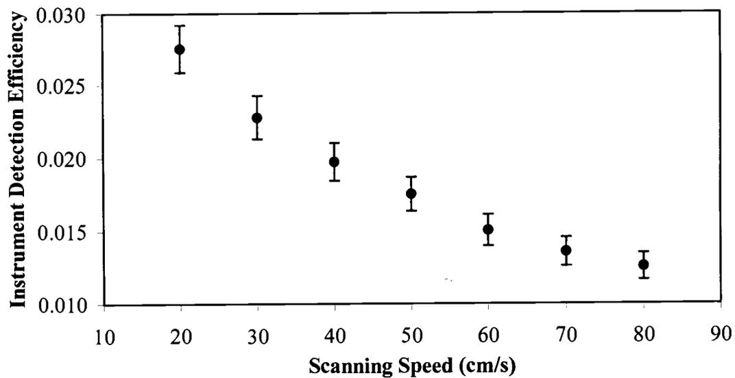
**Figure 7.** Experimentally determined values of 12.5 cm x 7.62 cm NaI(Tl) scintillator peak scanning instrument detection efficiency of 661.67 keV photons as a function of scanning speed. Error bars represent the 95% confidence interval, based on propagating the errors in counting statistics and in the measured source emission rate.
