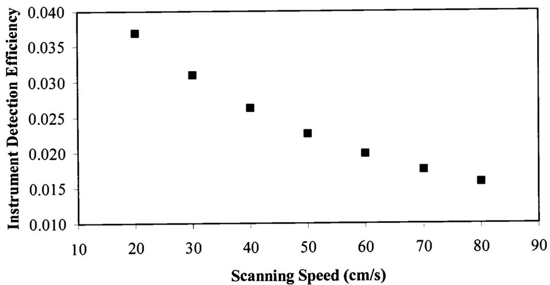
**Figure 5.** MCNP4b simulated 12.5 cm x 7.62 cm NaI(Tl) scintillator theoretical peak scanning instrument detection efficiency for 661.67 keV photons as a function of scanning speed.
