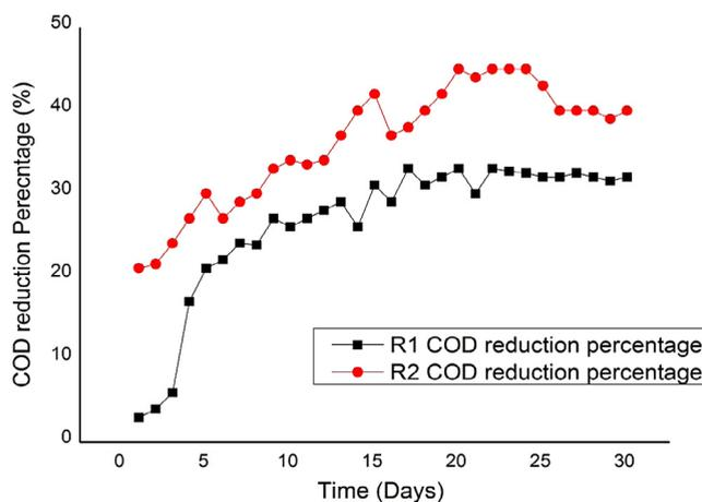
**Fig. 2.** COD reduction percentage of CSTR<sub>1</sub> and CSTR<sub>2</sub>. In figures CSTR<sub>1</sub> is shown as R<sub>1</sub> and CSTR<sub>2</sub> is shown as R<sub>2</sub>.
