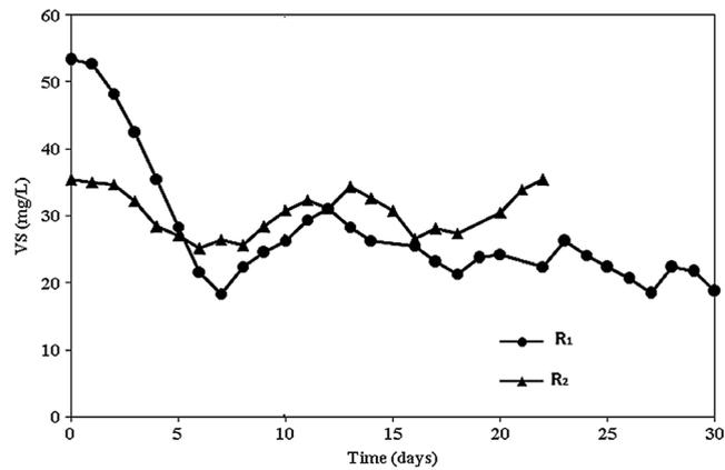
Fig. 3. VS concentrations in CSTR<sub>1</sub> and CSTR<sub>2</sub> during anaerobic digestion. In figures CSTR<sub>1</sub> is shown as R<sub>1</sub> and CSTR<sub>2</sub> is shown as R<sub>2</sub>.
