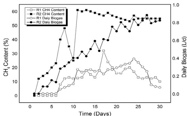
Fig. 1. Daily biogas production and methane content of the CSTR<sub>1</sub> and CSTR<sub>2</sub>. In figures CSTR<sub>1</sub> is shown as R<sub>1</sub> and CSTR<sub>2</sub> is shown as R<sub>2</sub>.
