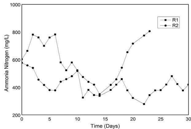
Fig. 4. Ammonia-nitrogen concentrations in CSTR<sub>1</sub> and CSTR<sub>2</sub> during anaerobic digestion. In figures CSTR<sub>1</sub> is shown as R<sub>1</sub> and CSTR<sub>2</sub> is shown as R<sub>2</sub>.
