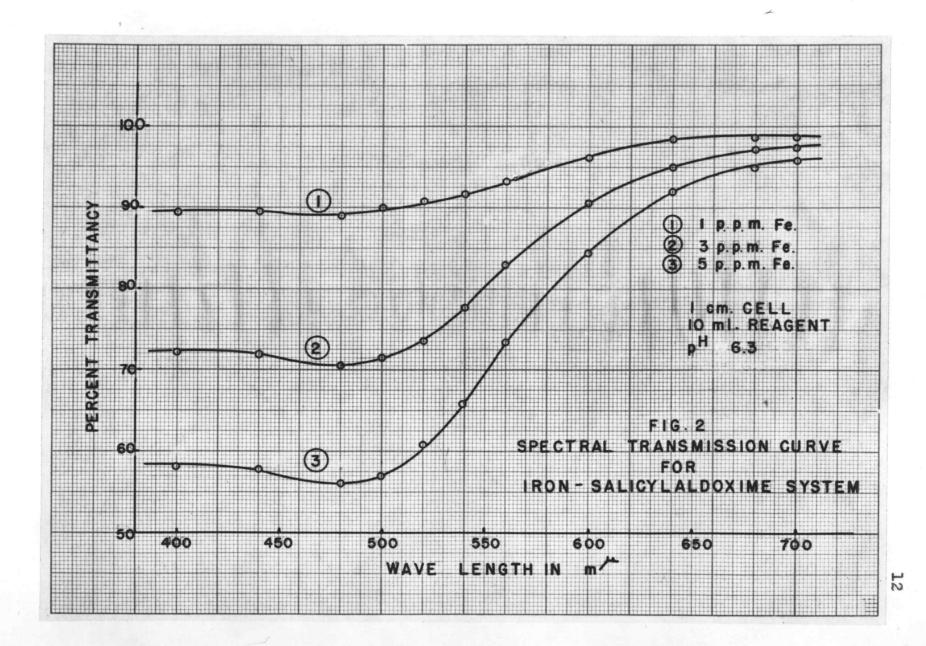
Again, the criterion for interference was the ability to obtain duplicate transmittancy readings. Solutions containing the same concentration of iron, but varying amounts of reagents were used. It was found that as long as enough reagent was present to react with all the iron, no adverse effect was evident. This is in agreement with Howe and Mellon (6).
