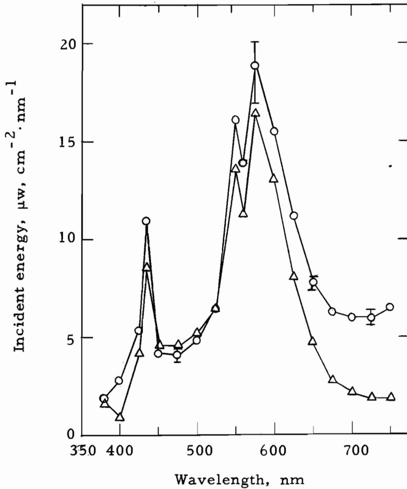
Figure 1. Spectral distribution of energy in the main (o) and auxiliary ( $\Delta$ ) growth chambers. Vertical bars denote the range of individual chamber measurements about the mean for the four main chambers.
