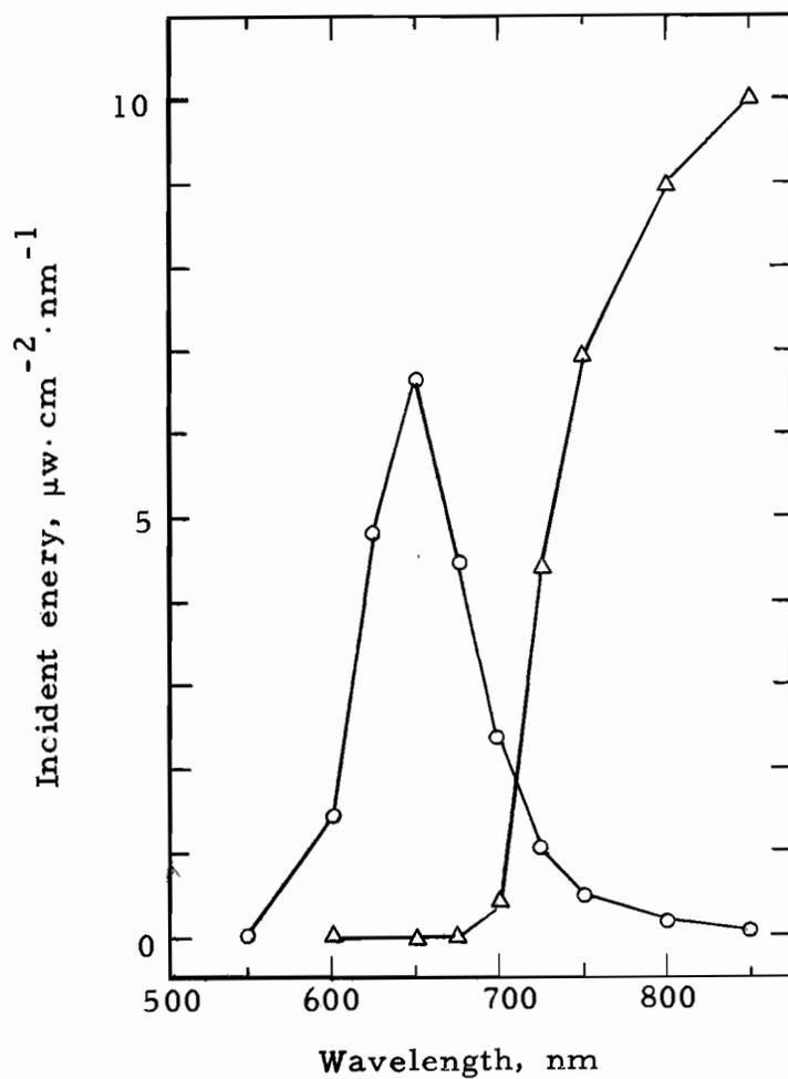
Figure 2. Spectral properties of the red (o) and far-red ( $\Delta$ ) light sources.
