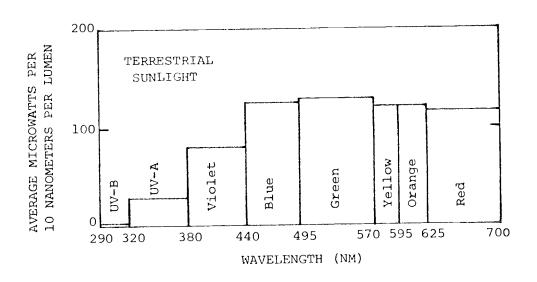
Fig. 3. Spectral energy distribution charts for Vita-Lite fluorescent lamps and terrestrial sunlight. The charts show the average amount of radiation generated in each color band by the source being measured. Charts are based on information supplied by the Duro-Test Corporation, North Bergen, New Jersey.
