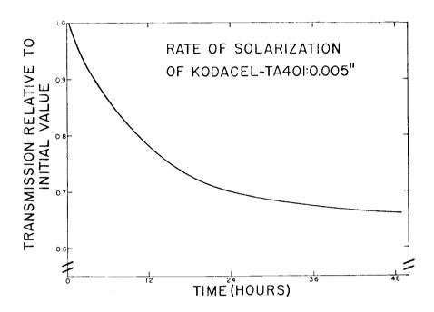
Figure 5. Effect of solarization on the transmission of Kodacel-TA401:0.005" in the UV-B region. Four FS40 sunlamps used as solarization source. Exposure rate without filter: three Sunburn Units per hour as measured with a UV-B Meter.
