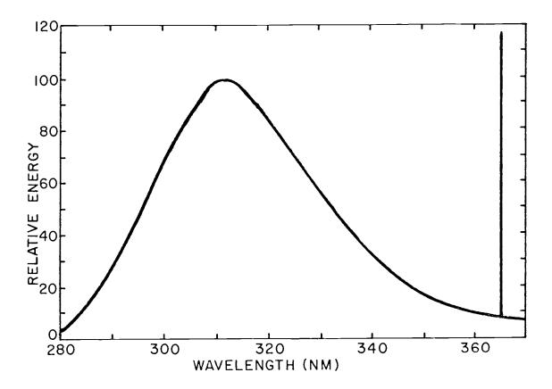
Figure 4. Emission spectrum of Westinghouse-FS40 fluorescent sunlamp. Closely spaced major emission lines of mercury at 366 nm are prominent, and are denoted as a single line. Spectrum based on information supplied by Westinghouse Electric Corporation.
