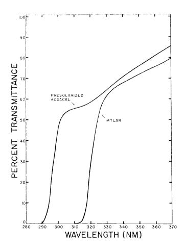
Figure 6. Transmission spectra for 0.13 mm thicknesses of 24-hour presolarized Kodacel-TA401:0.005" and nonsolarized Mylar 'S':0.005". This figure illustrates the transmission "window" between these two filters in the UV-B (290-315 nm) region.
