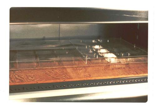
Figure 7. A group of eighteen culture dishes arranged on shelf of exposure apparatus, with nine dishes under Kodacel-TA401:0.005" and nine under Mylar 'S':0.005". Two sides of acrylic filter frame are raised to allow for ventilation.
