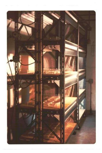
Figure 2. Exposure apparatus with protective side shielding removed for photographic purposes. Each shelf is 122 cm x 79 cm and has four two-lamp fluorescent fixtures located at 38 cm above the shelf. The outer lamp reflectors are asymmetric to optimize field homogeneity.
