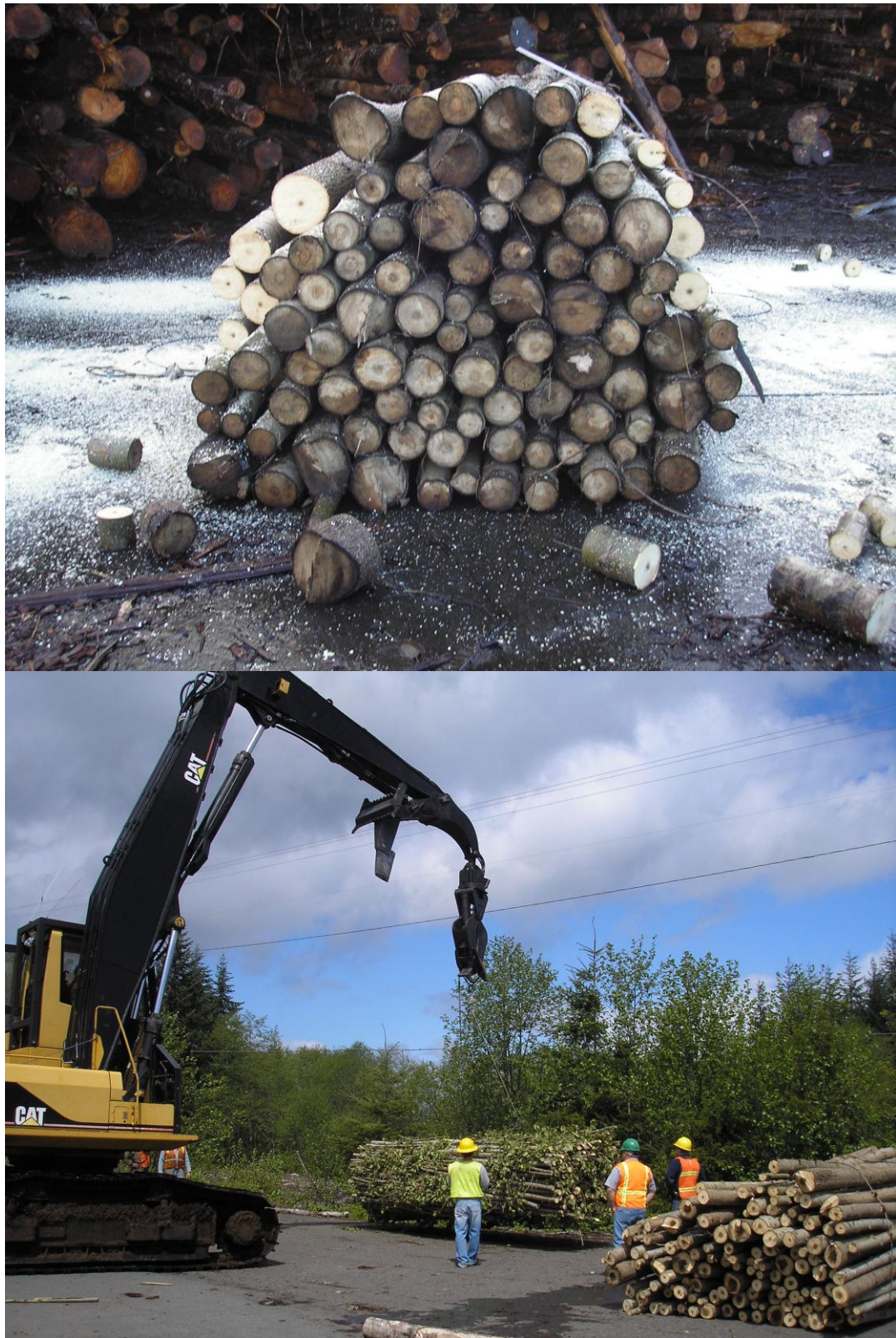
Figure A.3 Cross section of the large hybrid poplar bundle (above) and weighing a small hybrid poplar bundle using a crane scale and large hydraulic loader (bottom)
