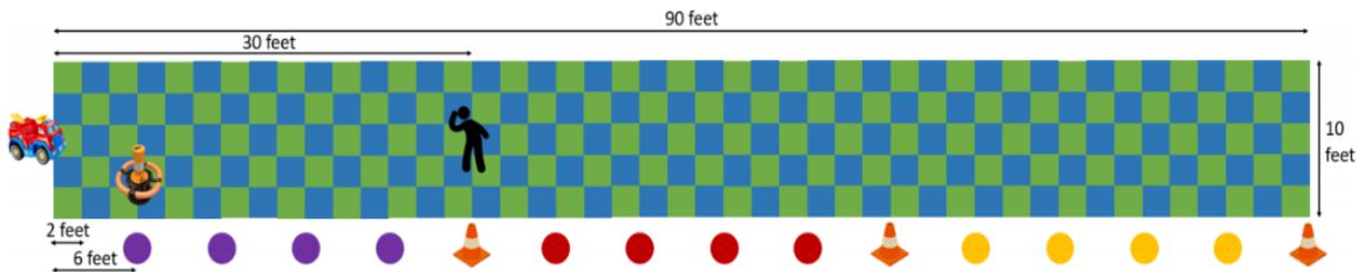
driving course on a gym floor. Poly spots were placed on the side of the course in 6-foot increments and three separate orange cones were placed along the course at 30 feet, 60 feet and 90 feet. This course, shown in figure 3 below, allowed researchers to easily measure driving distance and keep consistency with robot interactions.
