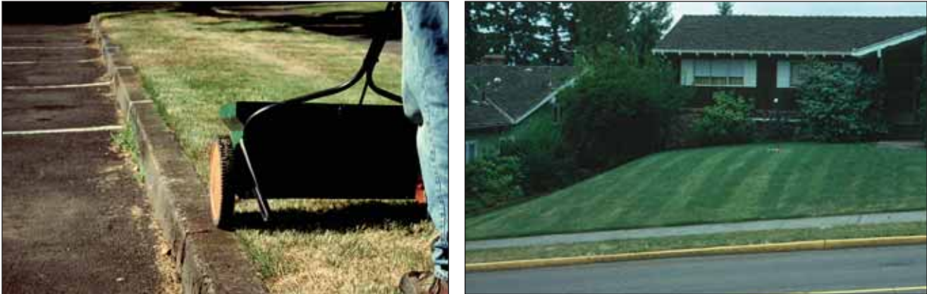
Figure 6. Drop spreaders are very accurate but must be operated properly. The lawn on the right has stripes because the operator failed to overlap each pass. You could say it got a half-rate application!
