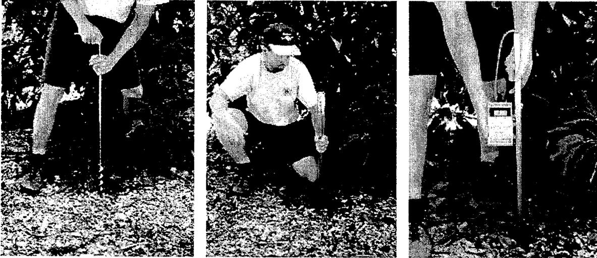
**Figure 4.** Installation and use of the Aqua-Pro high frequency dielectric moisture monitoring system. Careful installation is critical to accuracy of the readings.
