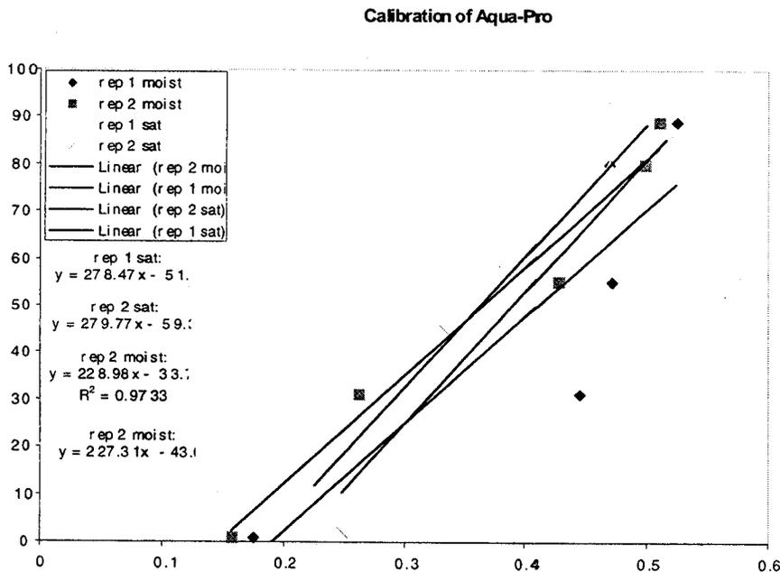
**Figure 5:** Preliminary calibration results for the Aqua-Pro sensor system as obtained in packed sand samples. The linearity and consistency of the data is encouraging. In addition, we have field data from the study which shows the same slope, with an off-set. Given the basic requirement of being able to track changes in water content in time, this data suggests that the system will be viable in vineyard irrigation management.
