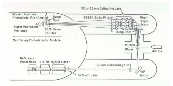
Figure 1. Diagram of FSSP instrument (Dye & Baumgardner, 1984).
