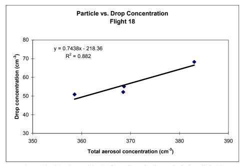
Figure 10. CONCF vs. CONCP from all passing intervals during Flight 18.
