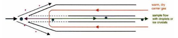
Figure 2. Diagram of CVI instrument (Twohy et al., 2003).
