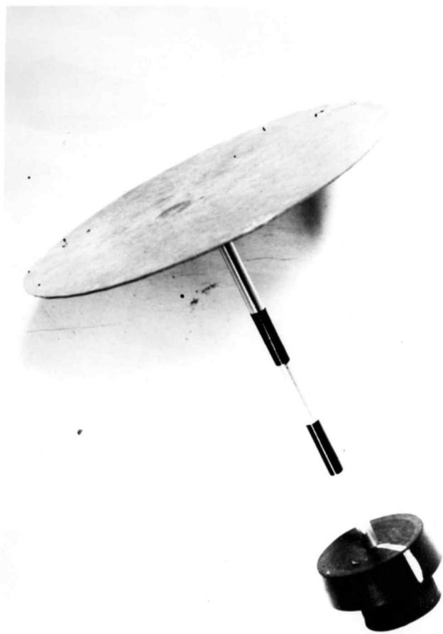
in two places, indicated by black bands in Figure 3, with clear cellophane tape (3/4 inch width). The two ends of the tape just met. With the tapes in place, rods were dipped in molten glycerin jelly. After allowing the excess glycerin jelly to drain, the rods were placed in cardboard mailing tubes until time for exposure.
