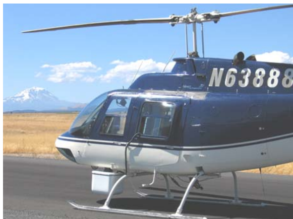
Figure 2 – Bell Jet Ranger equipped with a thermal infrared radiometer and high resolution digital camera. The sensors are contained in a composite fiber enclosure attached to the
