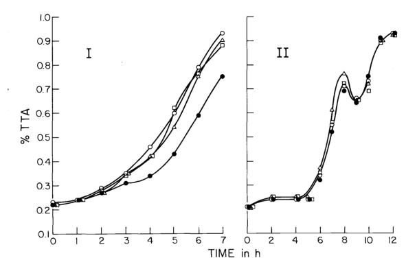
Fig. 2. TTA of 11% NFM cultures inoculated (1%) from 1.5 month old (I) or 7-8 month old (II) frozen (-20 C) concentrated multiple strain starter culture A infected with phages homologous for each component strain. O, uninfected control; □, infected with phage a1; △, infected with phage a2; ●, infected with phage a3. Data plotted were averaged from four experiments.
