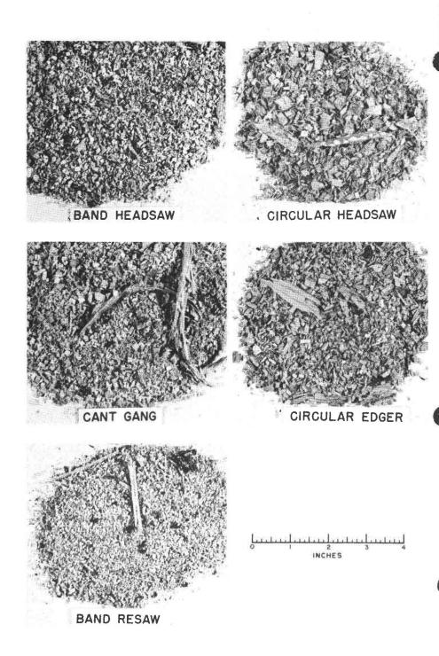
Figure 1. Representative samples of Douglas-fir sawdust collected from various saws.
