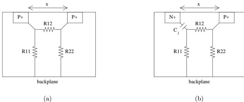
FIGURE 2.1. Lumped substrate model. (a) p+ to p+ model. (b) n+ to p+ model.
