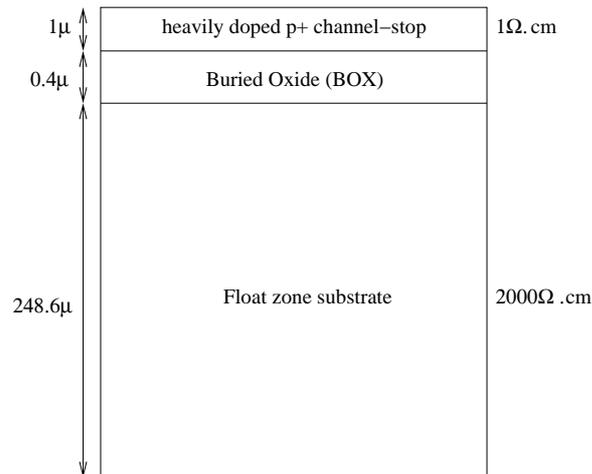
FIGURE 2.4. Cross-section of the SOI substrate (RF process).
