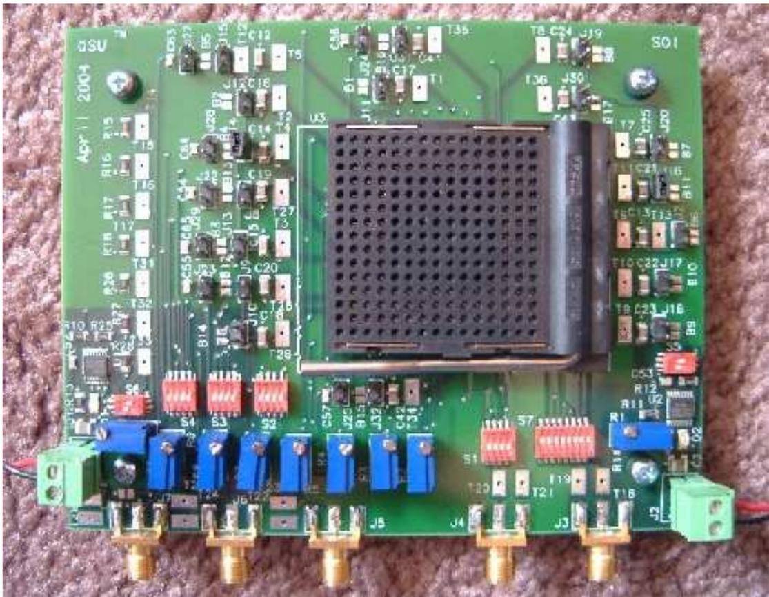
FIGURE D-18. Photo of SOI PCB test board.
