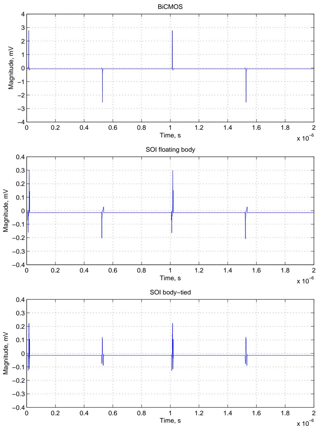
FIGURE 6.7. Noise picked up by a  $30\mu\text{m} \times 30\mu\text{m}$  sensor contact placed  $70\mu\text{m}$  away from the seventh stage of the stepped buffer in the BiCMOS process (top), the SOI process with floating body transistors (middle) and with body-tied transistors (bottom) and a clock frequency of 1MHz.
