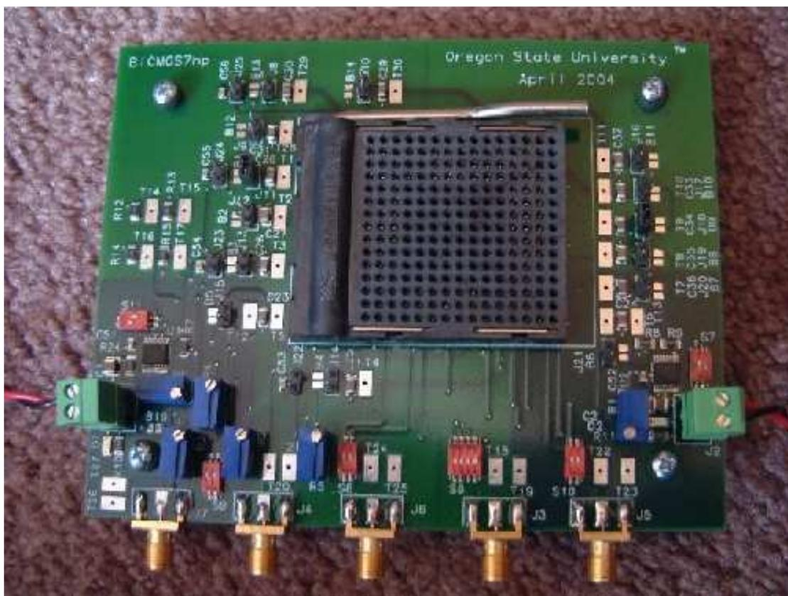
FIGURE D-15. Photo of BiCMOS PCB test board.
