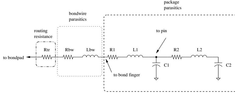
FIGURE 4.4. Package pin, bondwire, and routing resistance model.
