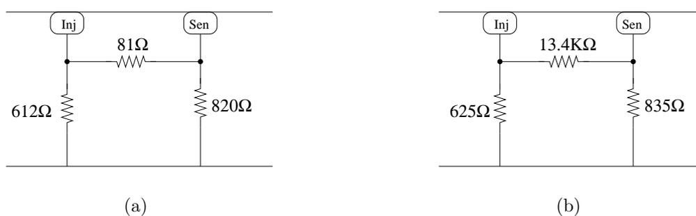
FIGURE 4.3. Resistive substrate network for  $30\mu\text{m} \times 30\mu\text{m}$  sensor and  $50\mu\text{m} \times 50\mu\text{m}$  injector contacts separated by  $100\mu\text{m}$ . (a) With buried layer. (b) Without buried layer.
