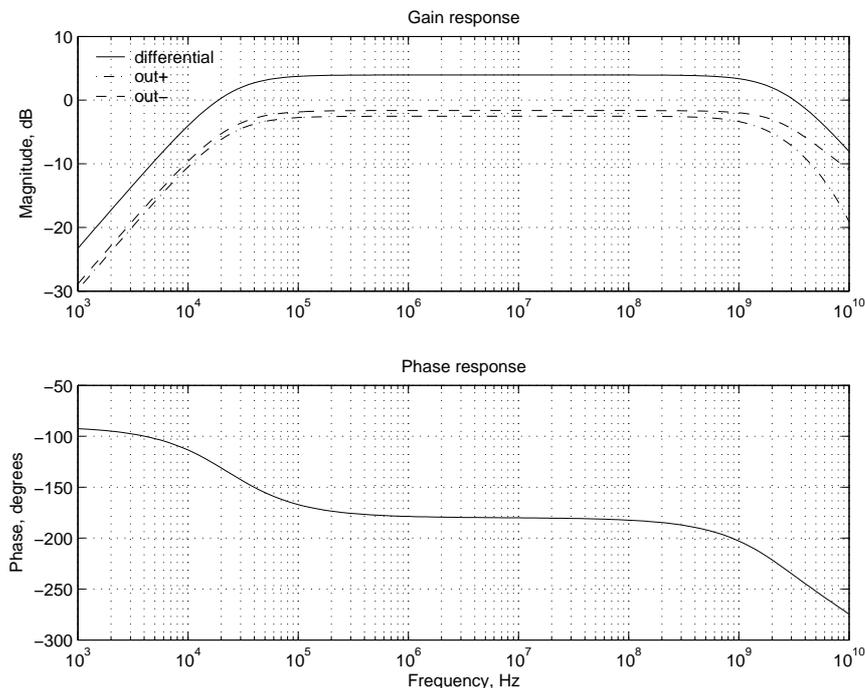
FIGURE 3.5. Differential gain and phase responses for *amp1*.
