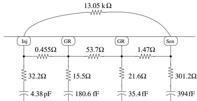
FIGURE 7.4. BiCMOS substrate network for a  $1\text{mm}^2$  contact and a  $0.09\text{mm}^2$  contact with  $10\mu\text{m}$  wide guard rings spaced at  $200\mu\text{m}$  around both contacts (spaced at  $240\mu\text{m}$ ).
