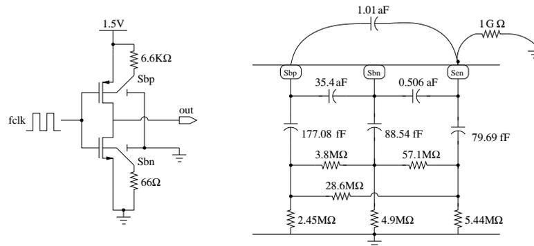
FIGURE 6.5. SOI body-tied transistor substrate network for the seventh stage of the stepped buffer and a  $30\mu\text{m} \times 30\mu\text{m}$  sensor contact placed  $70\mu\text{m}$  away, where Sbp and Sbn are the bulk terminals of the p-channel and n-channel transistors, respectively, and Sen is the sensor contact.
