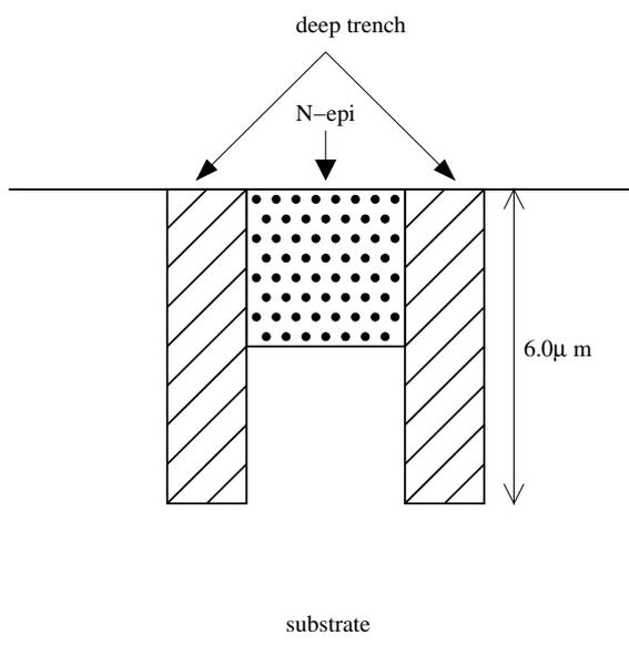
FIGURE 3.7. Cross-section of the deep trench moat.
