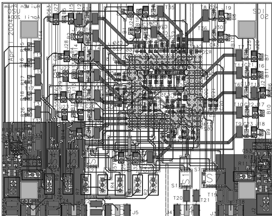
FIGURE D-17. Layout of SOI PCB test board.
