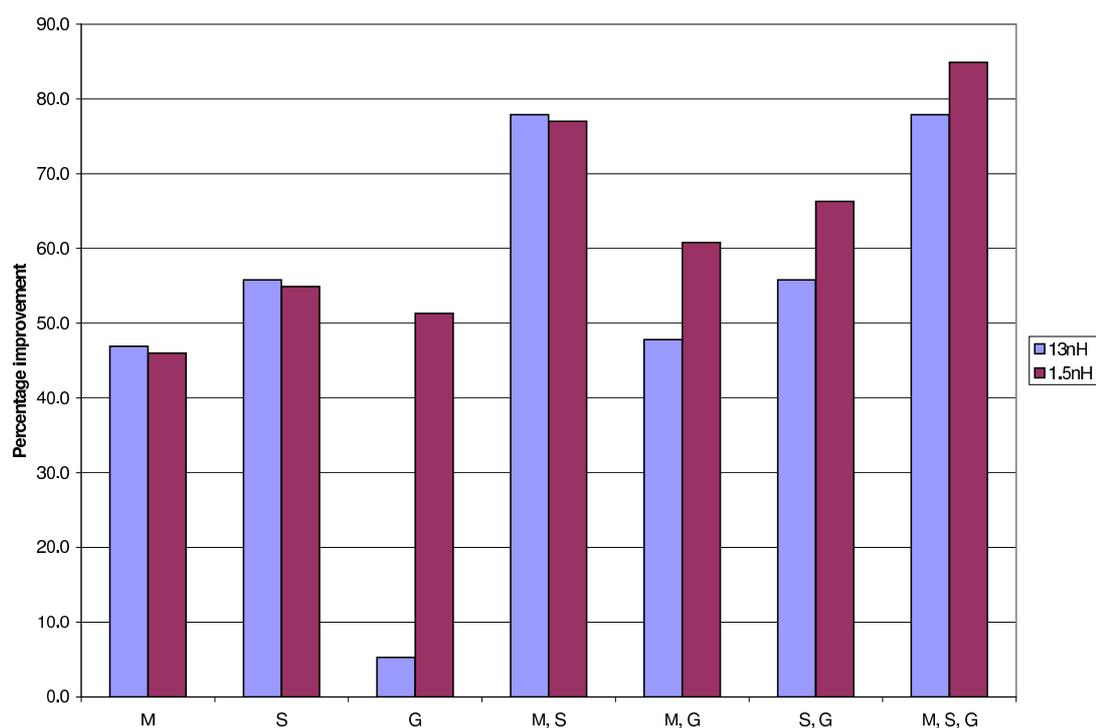
FIGURE 5.12. Comparison of noise suppression techniques in the  $0.18\mu\text{m}$  lightly doped BiCMOS process for 7 cases with a ground trace inductance of 13nH (light shading) and 1.5nH (dark shading), where M is the case with a moat, S is the case with the bulks and sources separated, and G is the case with the DPR grounded.
