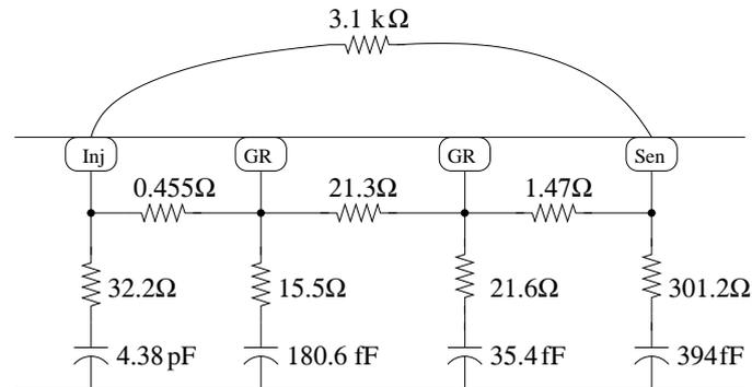
FIGURE 7.5. BiCMOS substrate network for a  $1\text{mm}^2$  contact and a  $0.09\text{mm}^2$  contact with  $10\mu\text{m}$  wide guard rings spaced at  $50\mu\text{m}$  around both contacts (spaced at  $90\mu\text{m}$ ).
