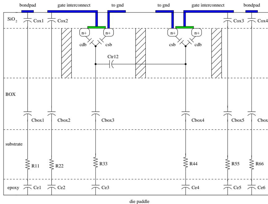
FIGURE 6.3. Generic SOI floating-body transistor substrate network example.
