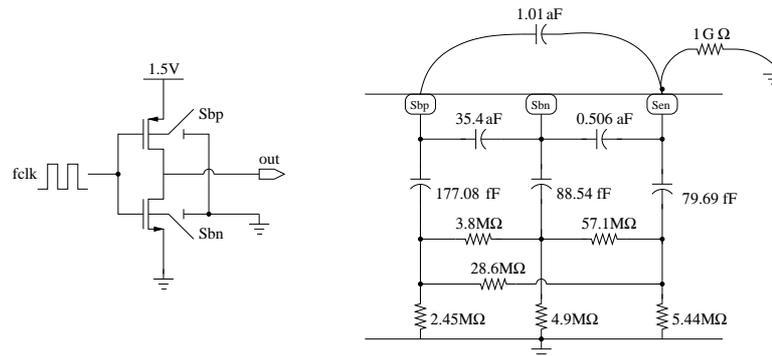
FIGURE 6.4. SOI floating-body transistor substrate network for the seventh stage of the stepped buffer and a  $30\mu\text{m} \times 30\mu\text{m}$  sensor contact placed  $70\mu\text{m}$  away, where Sbp and Sbn are the bulk terminals of the p-channel and n-channel transistors, respectively, and Sen is the sensor contact.
