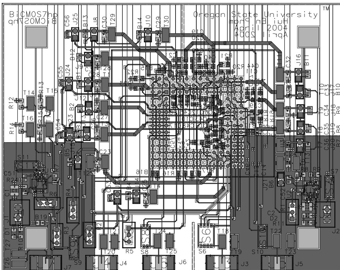
FIGURE D-13. Layout of BiCMOS PCB test board.
