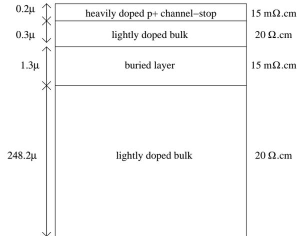
FIGURE 2.3. Typical cross-section of a lightly doped substrate with a buried layer.
