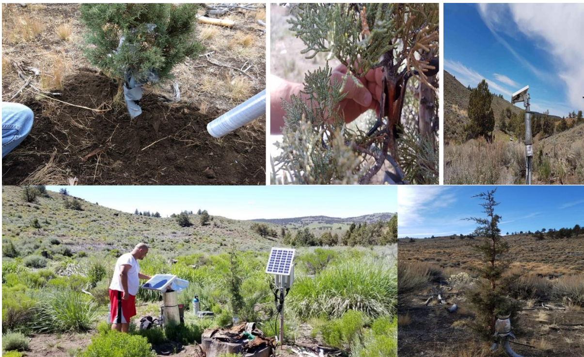
Figure A4.1. Installation of automated water use equipment in the field for the area (treated watershed) where small sapling trees that result after regrowth dominate.
