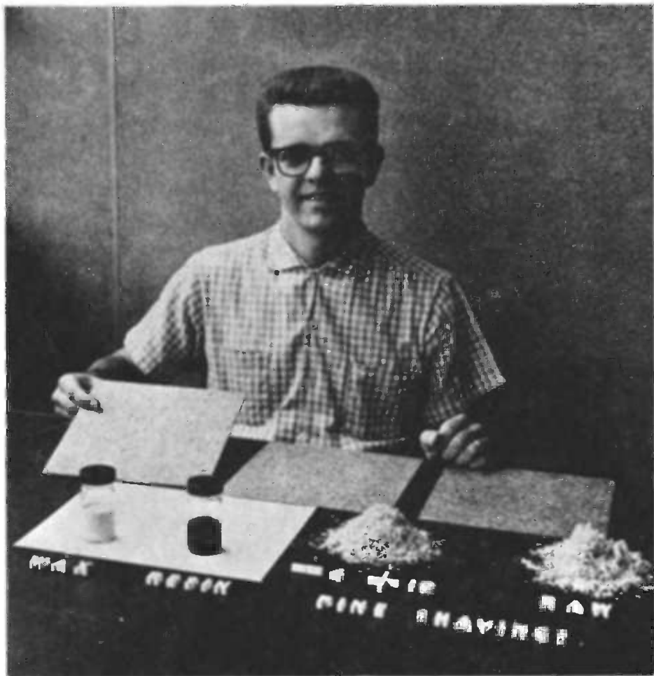
FLOOR TILE held by the author was made from screened hammer-milled planer shavings, wax, and resin, as shown in foreground.
