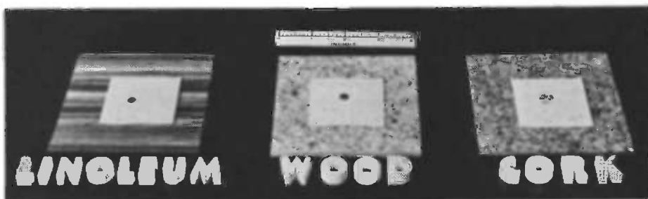
Figure 7. Diameter of mark left by carbon paper indicated extent of indentation in drop-ball test.
