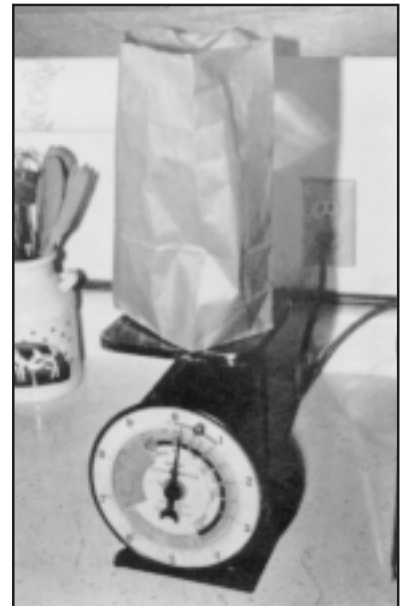
Figure 3.—Weigh your sample again. Repeat the drying and weighing until your sample's weight doesn't change.
