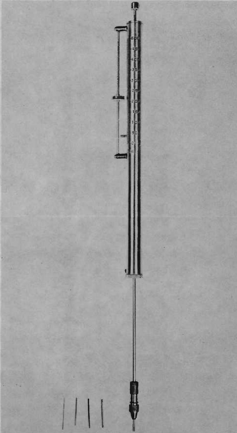
Figure 2. Texture tester equipped with various sizes of steel points.
