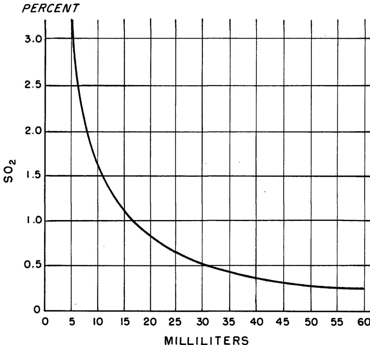
Figure 1. Milliliters of SO<sub>2</sub> required for 25 milliliters of 0.2 normal iodine solution.
