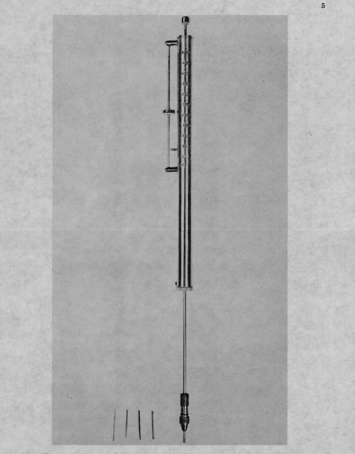
Figure 2. Texture tester equipped with various sizes of steel points.
